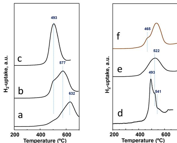
Fig. 4 H<sub>2</sub>-uptake during the TPR-H<sub>2</sub> experiments for activated catalysts: a) P8-N; b) P10-N; c) P11-N; d) P11A-N; e) P11B-N; f) P11C-aN. Characteristics of the catalysts are shown in Table 1.
