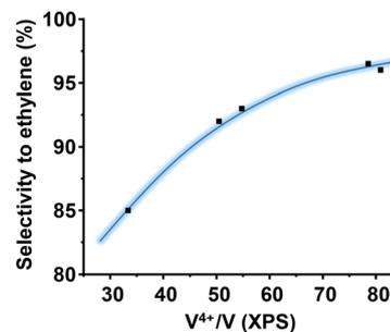
Fig. 8 Variation of the selectivity to ethylene during the ethane ODH with the  $\text{V}^{4+}$  content on the catalyst surface, determined by XPS. Reaction conditions for ethane ODH: 25% ethane conversion and a reaction temperature of 412 °C, and remaining conditions in the text.
