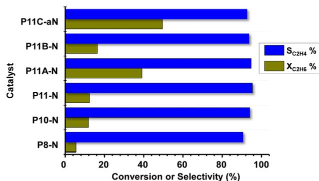
Fig. 7 Variation of ethane conversion ( $X_{C_2H_6}$ , %) and selectivity to ethylene ( $S_{C_2H_4}$ , %) during the ethane ODH over MoVTeNbO catalysts at a reaction temperature of 400 °C. Experimental conditions in the text.
