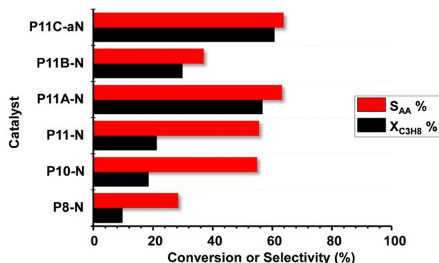
Fig. 6 Variation of propane conversion ( $X_{C_3H_8}$ , %) and selectivity to acrylic acid ( $S_{AA}$ , %) during partial oxidation of propane over MoVTeNbO catalysts at a reaction temperature of 380 °C. Experimental conditions in the text.
