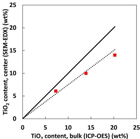
Fig. 4 Correlation of the bulk  $\text{TiO}_2$  content (measured by ICP-OES) and the semi-quantitative  $\text{TiO}_2$  content near the centre of the particles (determined by SEM-EDX) for samples overcoated with 1, 2 and 3 ALD cycles. The lines are meant to guide the eye and represent 100% parity (solid) and 75% parity (round dot) respectively.
