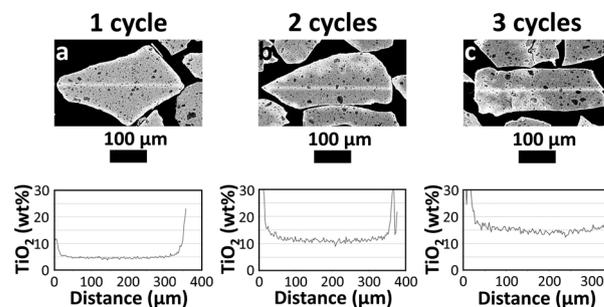
**Fig. 3** SEM-EDX line scans showing the TiO<sub>2</sub> distribution along the cross-section of the TiO<sub>2</sub>-Al<sub>2</sub>O<sub>3</sub> particles after 1, 2 and 3 TTIP ALD cycles (a, b and c, resp.). The location of the line scan is evident in the images as a brighter line across the length of the selected particle.
