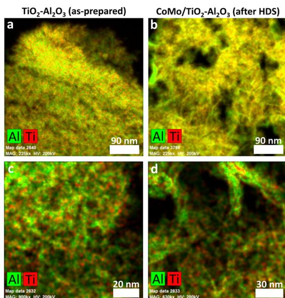
Fig. 7 Distribution of Al and Ti in a representative TiO<sub>2</sub>-Al<sub>2</sub>O<sub>3</sub> catalyst support (7.3 wt% TiO<sub>2</sub>, a and c) and a spent CoMo catalyst supported on the overcoated TiO<sub>2</sub>-Al<sub>2</sub>O<sub>3</sub> catalyst support (7 wt% TiO<sub>2</sub>, b and d) assessed by TEM-EDX. Red: Ti; green Al.
