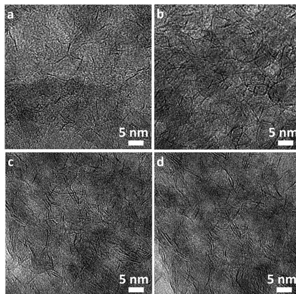
Fig. 8 High resolution TEM images on several sample locations (a–d) of a spent overcoated CoMoS catalyst (7 wt% TiO<sub>2</sub> after 1 TTIP ALD cycle) obtained after the catalytic performance testing.
