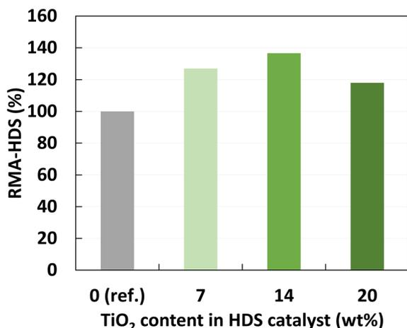
Fig. 6 HDS activity (RMA) of TiO<sub>2</sub>-Al<sub>2</sub>O<sub>3</sub> supported CoMo catalysts. The Al<sub>2</sub>O<sub>3</sub> support was overcoated with 1, 2 and 3 TTIP ALD cycles resulting in 7, 14 and 20 wt% TiO<sub>2</sub> respectively. For benchmarking, the activity of the analogous reference catalyst without a TiO<sub>2</sub> overcoating is included.
