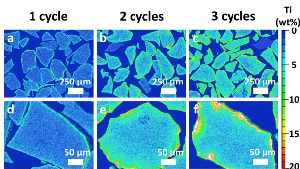
**Fig. 2** Titanium distribution (determined by SEM-EDX) inside the TiO<sub>2</sub>-Al<sub>2</sub>O<sub>3</sub> particles after 1, 2 and 3 TTIP ALD cycles: (a–c) low and (d–f) high magnifications respectively. White colour indicates a very high (>20 wt%) local Ti content.
