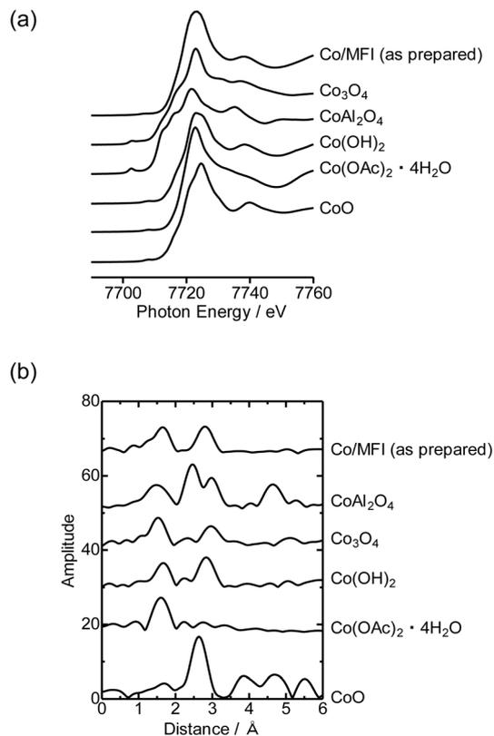
Fig. 1 Co K-edge (a) XANES and (b) EXAFS-FT of Co/MFI(52N) (Co: 0.5 mmol g<sup>-1</sup>) and reference compounds measured at 298 K. Fourier transform range: 3–13 Å<sup>-1</sup>.
