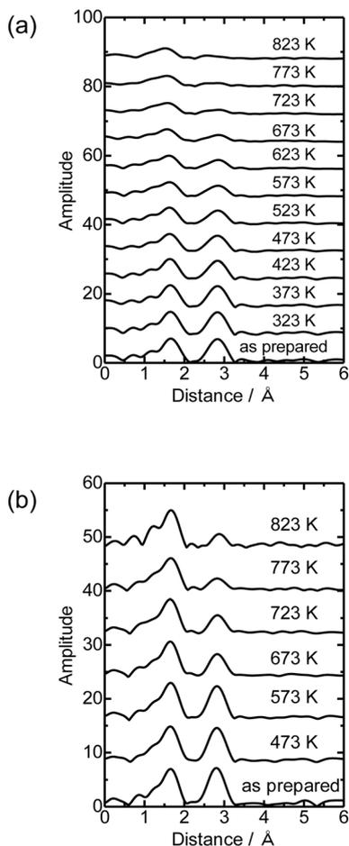
**Fig. 4** Co K-edge EXAFS-FT of Co/MFI(52N) (Co: 0.5 mmol g<sup>-1</sup>) (a) measured under a N<sub>2</sub> flow from 323 to 823 K under *in situ* conditions, the as-prepared sample and (b) measured under ambient conditions.
