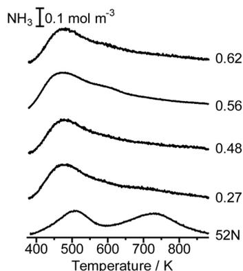
Fig. 5  $\text{NH}_3$  TPD profile of unloaded MFI(52N) and Co/MFI(52N). The samples were treated in an  $\text{N}_2$  flow at 773 K prior to the TPD measurement. The numbers indicate the loading of Co ( $\text{mmol g}^{-1}$ ).
