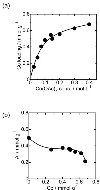
Fig. 2 (a) Relationship between the Co loading of Co/MFI(52N) and concentration of Co(OAc)<sub>2</sub>. (b) Relationship between Co loading and the Al concentration of Co/MFI(52N).
