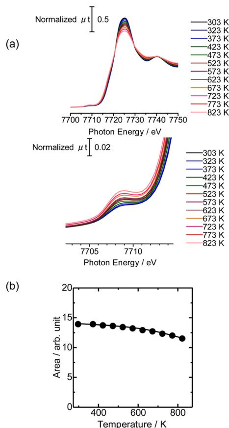
Fig. 3 (a) Co K-edge XANES of Co/MFI(52N) (Co: 0.5 mmol g<sup>-1</sup>) measured under a N<sub>2</sub> flow from 303 to 823 K measured under *in situ* conditions. (b) White line area in Co K-edge XANES of Co/MFI(52N) plotted as a function of the treatment temperature.
