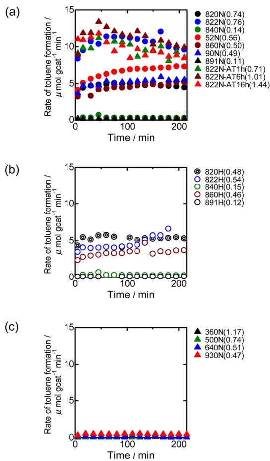
Fig. 9 Time course change of the toluene formation rate over Co loaded on different kinds of zeolite supports: (a)  $NH_4$ -form MFI, (b) H-form MFI, and (c) zeolites other than MFI. The Co/MFI catalysts were prepared using a  $200 \text{ mmol L}^{-1}$   $Co(OAc)_2$  solution at 343 K for 4 h. The numbers in the parentheses indicate the loading of Co ( $\text{mmol g}^{-1}$ ).
