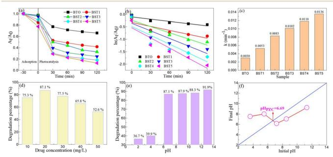
Fig. 8 (a) The degradation efficiency for TC-HCl on the BST photocatalysts. (b) Plots of  $\ln{(A_t/A_0)}$  vs. irradiation time of the BST photocatalysts for the degradation of TC-HCl. (c) The apparent degradation rate constant (k) value of the BST photocatalysts for the degradation of TC-HCl. Effects of (d) drug concentration and (e) pH value on the degradation of TC-HCl on the BST5 photocatalyst. (f) PZC of the BST5 photocatalyst.
