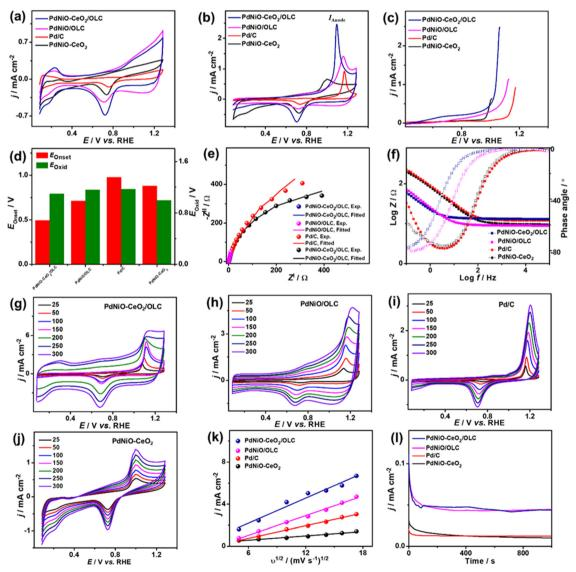
Fig. 3 CV profiles at 50 mV s<sup>-1</sup> in (a) N<sub>2</sub>-saturated HClO<sub>4</sub> (0.1 M) and (b) CO-saturated HClO<sub>4</sub> (0.1 M). (c) LSV at 50 mV s<sup>-1</sup>. (d)  $E_{Onset}$  and  $E_{Oxid}$ . (e) Nyquist plots. (f) Bode plots. (g-j) Scan rate studies. (k) Randles-Sevcik plots ( $I_{Anode}$  vs.  $v^{1/2}$ ). (l) CA of PdNiO-CeO<sub>2</sub>/OLC, PdNiO/OLC, PdNiO/OCC, PdNiO-CeO, and PdC in CO-saturated HClO<sub>4</sub> (0.1 M).
