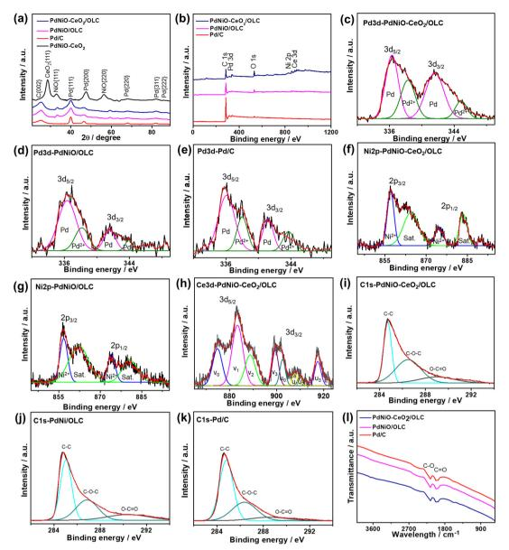
Fig. 2 (a) XRD patterns, (b) XPS wide-survey scans, high-resolution XPS spectra of (c-e) Pd3d, (f and g) Ni2p, (h) Ce3d, (i-k) C1s, and (l) FTIR spectra of PdNiO-CeO<sub>2</sub>/OLC, PdNiO/OLC, PdNiO-CeO<sub>2</sub>, and Pd/C nanocrystals.
