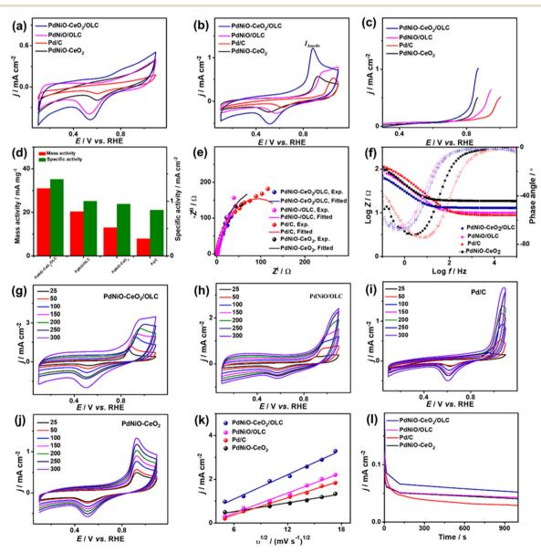
Fig. 5 CV profiles at 50 mV s<sup>-1</sup> in (a) N<sub>2</sub>-saturated NaHCO<sub>3</sub> (0.1 M) and (b) CO-saturated NaHCO<sub>3</sub> (0.1 M). (c) LSV at 50 mV s<sup>-1</sup>. (d) Mass/specific activities. (e) Nyquist plots. (f) Bode plots. (g-j) Scan rate studies. (k) Randles-Sevcik plots (I<sub>Anode</sub> vs. v<sup>1/2</sup>) and (l) CA of PdNiO-CeO<sub>2</sub>/OLC, PdNiO/ OLC, PdNiO-CeO<sub>2</sub>, and PdC in CO-saturated NaHCO<sub>3</sub> (0.1 M).
