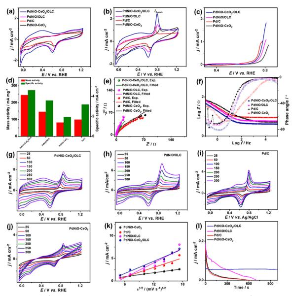
Fig. 4 CV curves at 50 mV s<sup>-1</sup> in (a) N<sub>2</sub>-saturated KOH (0.1 M) and (b) CO-saturated KOH (0.1 M). (c) LSV at 50 mV s<sup>-1</sup>. (d) Mass/specific activities. (e) Nyquist plots. (f) Bode plots. (g-j) Scan rate studies. (k) Randles-Sevcik plots ( $I_{Anode}$  vs.  $v^{1/2}$ ) and (l) CA of PdNiO-CeO<sub>2</sub>/OLC, PdNiO/OLC, PdNiO-CeO<sub>2</sub>, and Pd/C in CO-saturated KOH (0.1 M).
