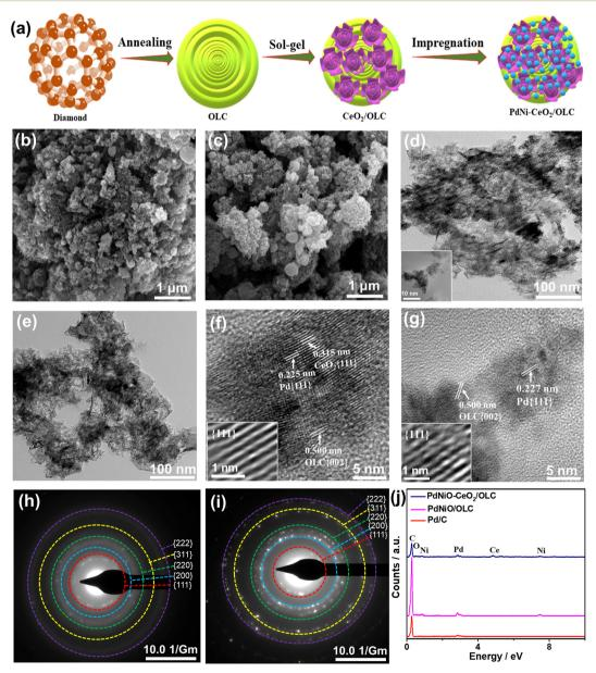
Fig. 1 (a) Schematic preparation method. (b and c) SEM images, (d and e) TEM micrographs, (f and g) HRTEM images with Fourier-transform HRTEM, and (h and i) SAED patterns of PdNiO-CeO<sub>2</sub>/OLC and PdNiO/OLC, respectively, and (j) EDX analysis.
