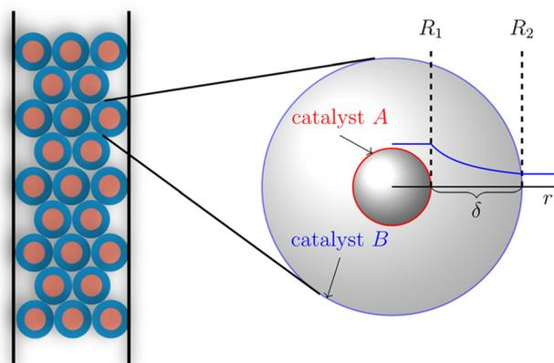
**Fig. 6** Core–shell catalyst with catalyst A as core catalyzing the methanol reaction with rate  $R_1$ . A shell with thickness  $\delta$  separates catalyst B from catalyst A. At catalyst B methanol is converted to DME at a rate  $R_2$ . The decaying curve represents the concentration profile of methanol as the intermediate product in this tandem reaction.
