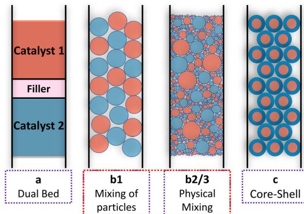
Fig. 5 Arrangement of bifunctional catalysts for CO<sub>2</sub> conversion. a) Dual catalyst bed without any mixing, b1) mechanical mixing of catalyst particles without applying external forces, b2) mixing in aqueous dispersions, b3) physical mixing of catalyst powders applying external forces (grinding, milling), c) chemical mixing by impregnation of core-shell particles.
