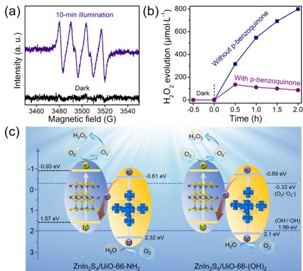
**Fig. 6** EPR spectra of DMPO- $\cdot\text{O}_2^-$  adducts using Z-UN at dark and 10 min illumination (a), photocatalytic  $\text{H}_2\text{O}_2$  evolution using Z-UN with and without *p*-benzoquinone (b), the proposed mechanism for photocatalytic  $\text{H}_2\text{O}_2$  evolution using Z-UN and Z-U(OH) $_2$  (c).
