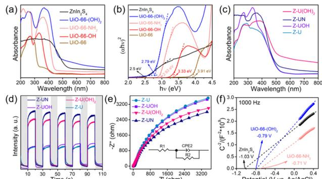
**Fig. 5** UV-vis DRS (a) and  $(\alpha hv)^2$  versus  $h\nu$  curves (b) of ZnIn<sub>2</sub>S<sub>4</sub>, UiO-66-(OH)<sub>2</sub>, UiO-66-NH<sub>2</sub>, UiO-66-OH and UiO-66, UV-vis DRS (c), photocurrent spectra (d) and EIS Nyquist plots (e) of Z-UN, Z-U(OH)<sub>2</sub>, Z-UOH and Z-U, Mott-Schottky plots of ZnIn<sub>2</sub>S<sub>4</sub>, UiO-66-(OH)<sub>2</sub> and UiO-66-NH<sub>2</sub> (f).
