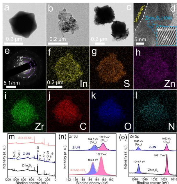
**Fig. 4** TEM images of UiO-66-NH<sub>2</sub> (a), ZnIn<sub>2</sub>S<sub>4</sub> (b) and Z-UN (c and d), SAED pattern (e) and EDS mapping images (f–l) of Z-UN, XPS spectra of UiO-66-NH<sub>2</sub>, Z-UN and ZnIn<sub>2</sub>S<sub>4</sub>: survey (m), Zr 3d (n) and Zn 2p (o).
