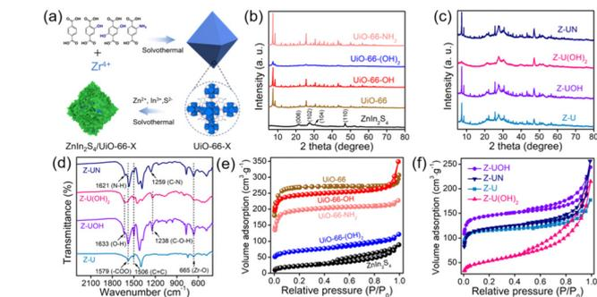
**Fig. 2** Preparation diagram of  $\text{ZnIn}_2\text{S}_4/\text{UiO-66-X}$  hybrids (a), XRD patterns (b and c) and  $\text{N}_2$  adsorption–desorption isotherms (e and f) of UiO-66- $\text{NH}_2$ , UiO-66- $(\text{OH})_2$ , UiO-66-OH, UiO-66,  $\text{ZnIn}_2\text{S}_4$ , Z-UN, Z-U( $\text{OH})_2$ , Z-UOH and Z-U, FTIR spectra of Z-UN, Z-U( $\text{OH})_2$ , Z-UOH and Z-U (d).
