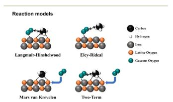
Fig. 2 Schematic diagram of the reaction mechanism of catalytic methane combustion. Reproduced from ref. 32 with permission from the American Chemical Society.
