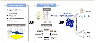
Fig. 15 Machine learning methodology for the discovery of Ag/MnO<sub>x</sub> catalysts consists of (i) experimental design, (ii) machine learning framework, (iii) composition exploration and prediction, and (iv) experimental verification and feedback. Reproduced from ref. 219 with permission from Elsevier.
