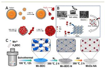
Fig. 14 (A) Scheme for the transformation process of the Co<sub>3</sub>O<sub>4</sub> catalyst. Reproduced from ref. 78 with permission from Springer Nature. (B) The preparation process of the MnO<sub>2</sub> catalyst by a combined ball-milling and selective atom removal method. Reproduced from ref. 209 with permission from Elsevier. (C) Preparation process of the MnO<sub>x</sub>-NA catalyst. Reproduced from ref. 210 with permission from the American Chemical Society.
