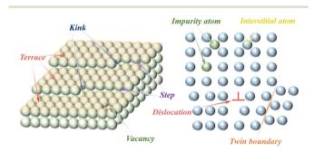
Fig. 4 Schematic illustrating the different types of defects in catalyst
