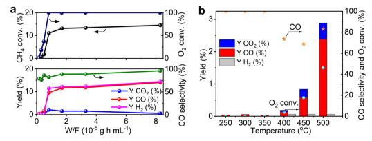
Fig. 5 Effect of contact time (a) and reaction temperature (b) on the POM over reduced Re/MOR. CH<sub>4</sub>: O<sub>2</sub>: N<sub>2</sub> = 50:4:46. Detailed reaction data for (a) are available in Table S2.†
