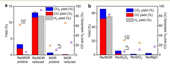
Fig. 3 POM over different catalysts. (a) Re/MOR and MOR before and after  $H_2$  reduction (600 °C). Reaction conditions: 600 °C,  $CH_4: O_2: N_2 = 50:4:46$ , space velocity (SV) of 60 000 mL  $g^{-1}$  h<sup>-1</sup>. (b) Effect of catalyst support. Catalysts were reduced before POM. 600 °C,  $CH_4: O_2: N_2 = 8:4:88$ , SV of 12 000 mL  $g^{-1}$  h<sup>-1</sup>. All the data in (a) and (b) are results at 1 h after starting the reaction.
