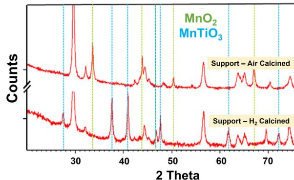
Fig. 4 XRD of the *ex situ* prepared catalyst supports composed of only titania and manganese (90:10). The air-calcined material formed only MnO<sub>2</sub>, while that calcined in hydrogen formed the MnTiO<sub>3</sub> phase. Other peaks (unmarked) are due to TiO<sub>2</sub> phases.
