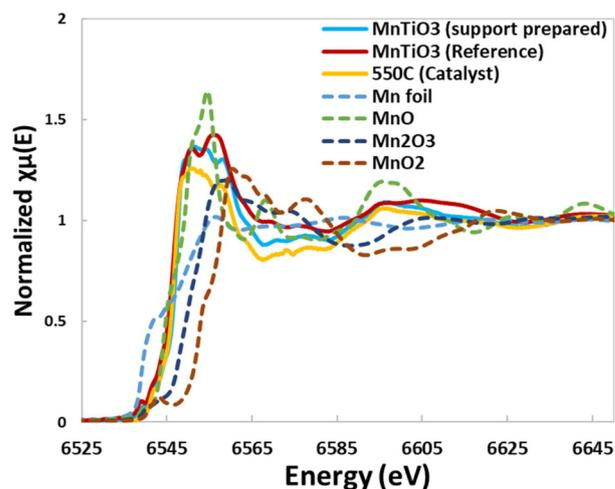
**Fig. 6** XAS data from XANES showing the close correlation of the synthesised material with the MnTiO<sub>3</sub> standard and the EXAFS data fitting the theoretical structure.
