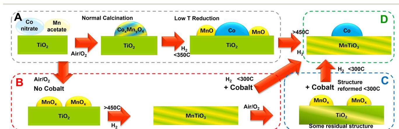
**Fig. 9** Summary of the transitions seen for manganese following high or low temperature reductions in air and hydrogen. Initially starting with cobalt and manganese precursors with the titania support (A), the catalyst can be reduced at elevated temperatures to make cobalt metal on MnTiO<sub>3</sub> (D). Alternatively, a preformed support material can be synthesized from manganese and titania (B) and cobalt can be added later without exposing the cobalt to a high reduction temperature (C).
