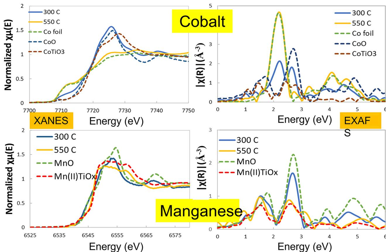
**Fig. 3** X-ray Absorption Spectroscopy (XAS) at the cobalt and manganese edges. EXAFS and XANES data are shown following treatments at 300 °C (solid blue lines) and 550 °C (solid yellow lines) with standard reference measurements provided as the dashed lines.
