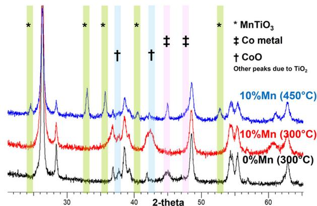
Fig. 2 *In situ* XRD of CoTiO<sub>2</sub> with 0 and 10% Mn during reduction in 100% H<sub>2</sub>. The formation of a titanate phase with ABO<sub>3</sub> structure is seen at 450 °C for the high manganese loaded catalyst.
