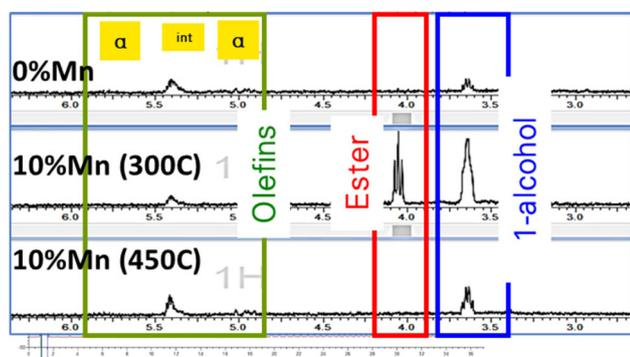
Fig. 1 Product wax analysis by <sup>1</sup>H NMR for 10% Co/TiO<sub>2</sub> catalysts with and without manganese promoter following reduction at 300 °C (for 0% Mn) and at 300 °C and 450 °C for 10% Mn.
