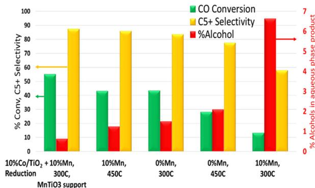
**Fig. 8** A summary of the reactor testing data for the different catalysts (with/without 10% Mn) and the activation temperature. The highest activity and selectivity was achieved for the pre-prepared MnTiO<sub>3</sub> supported catalyst, while the conventional Co/Mn/TiO<sub>2</sub> catalyst exhibits increased selectivity to higher alcohols.
