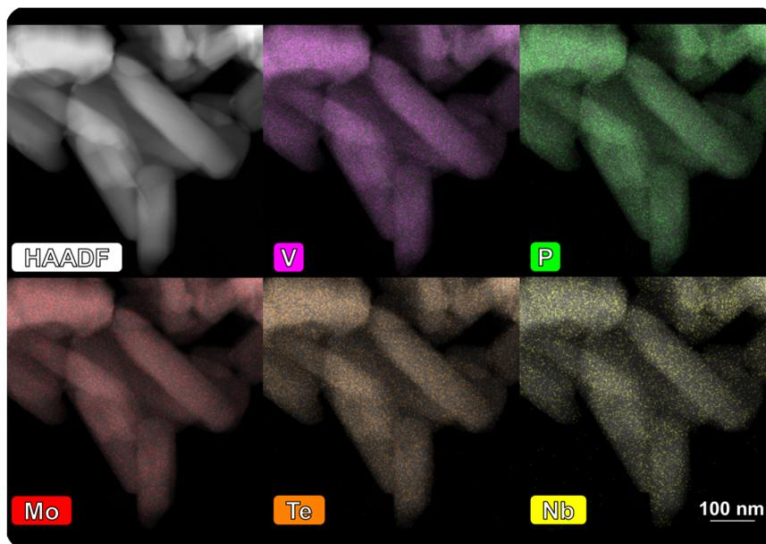
Fig. 3 STEM-HAADF images of  $\text{PO}_x$  surface-modified  $\text{MoVTeNbO}_x$  after catalysis (spent sample): EDX-mappings show element dispersion of both bulk elements (Mo, V, Te, Nb) and the additionally deposited phosphorus; the images of the fresh sample are shown in Fig. S18;† the mapping-spectra of both samples are attached in Fig. S19 and S110.†
