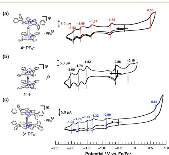
Fig. 5 Comparison of cyclic voltammograms of (a)  $4^+\cdot\text{PF}_6^-$ , (b)  $1^+\cdot\text{I}^-$ , and (c)  $3^+\cdot\text{PF}_6^-$  in a pyridine solution containing 100 mM of  $^n\text{Bu}_4\text{N}^+\cdot\text{PF}_6^-$  at room temperature. [Substrate] = 200  $\mu\text{M}$ , [scan rate] = 100  $\text{mV s}^{-1}$ .
