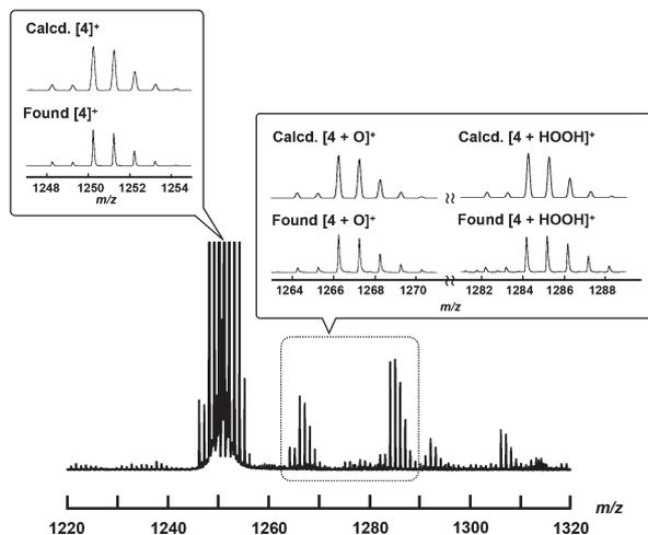
**Fig. 6** ESI-TOF MS spectrum of  $4^+ \cdot I_3^-$  in an aqueous  $CH_3CN$  solution containing excess amount of  $H_2O_2$  at room temperature (the detail of the experimental procedure is shown in the Experimental section). Insets: Comparison of calculated (top) and experimental (bottom) isotopic distribution patterns of molecular peaks assignable to  $[4]^+$ ,  $[4 + O]^+$ , and  $[4 + HOOH]^+$ .
