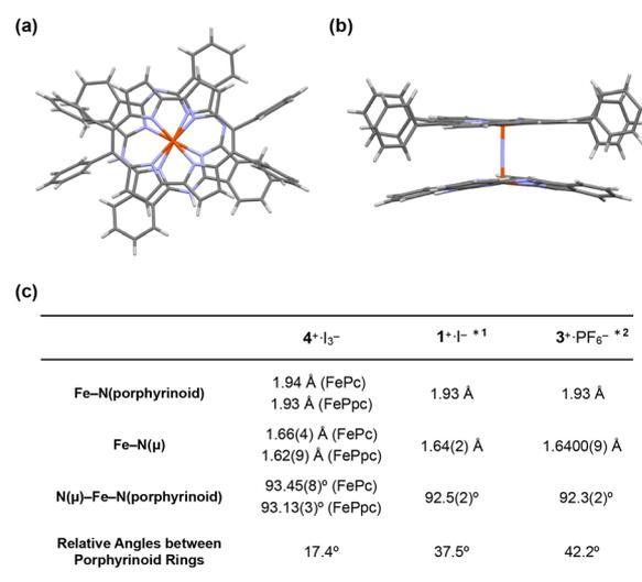
Fig. 4 (a) Side and (b) top views of the single crystal X-ray structure of  $4^+\cdot\text{I}_3^-$ .  $\text{I}_3^-$ , coordinating pyridines, and crystalline solvents were omitted for clarity. (c) Comparison of some mean bond lengths and angles of  $4^+\cdot\text{I}_3^-$ ,  $1^+\cdot\text{I}^-$ , and  $3^+\cdot\text{PF}_6^-$ . \*1: ref. 28, \*2: ref. 38.
