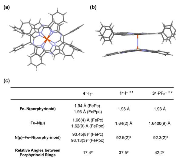
Fig. 4 (a) Side and (b) top views of the single crystal X-ray structure of  $4^+\cdot I_3^-$ .  $I_3^-$ , coordinating pyridines, and crystalline solvents were omitted for clarity. (c) Comparison of some mean bond lengths and angles of  $4^+\cdot I_3^-$ ,  $1^+\cdot I^-$ , and  $3^+\cdot PF_6^-$ . \*1: ref. 28, \*2: ref. 38.
