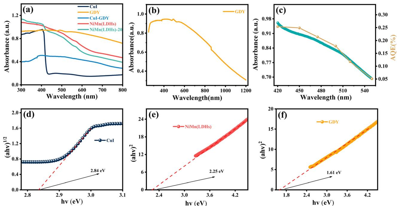
Fig. 7 (a) UV-vis diffuse reflectance spectra of CuI, GDY, CuI-GDY, NiMn(LDHs) and NiMn(LDHs)-20. (b) UV-vis diffuse reflectance spectra of GDY. (c) The apparent quantum efficiency of  $H_2$  evolution for NiMn(LDHs)-20 under irradiation at different wavelengths (right axis), and the corresponding ultraviolet-visible spectrum (left axis) (d–f) and band gap energies of CuI, NiMn(LDHs) and GDY.
