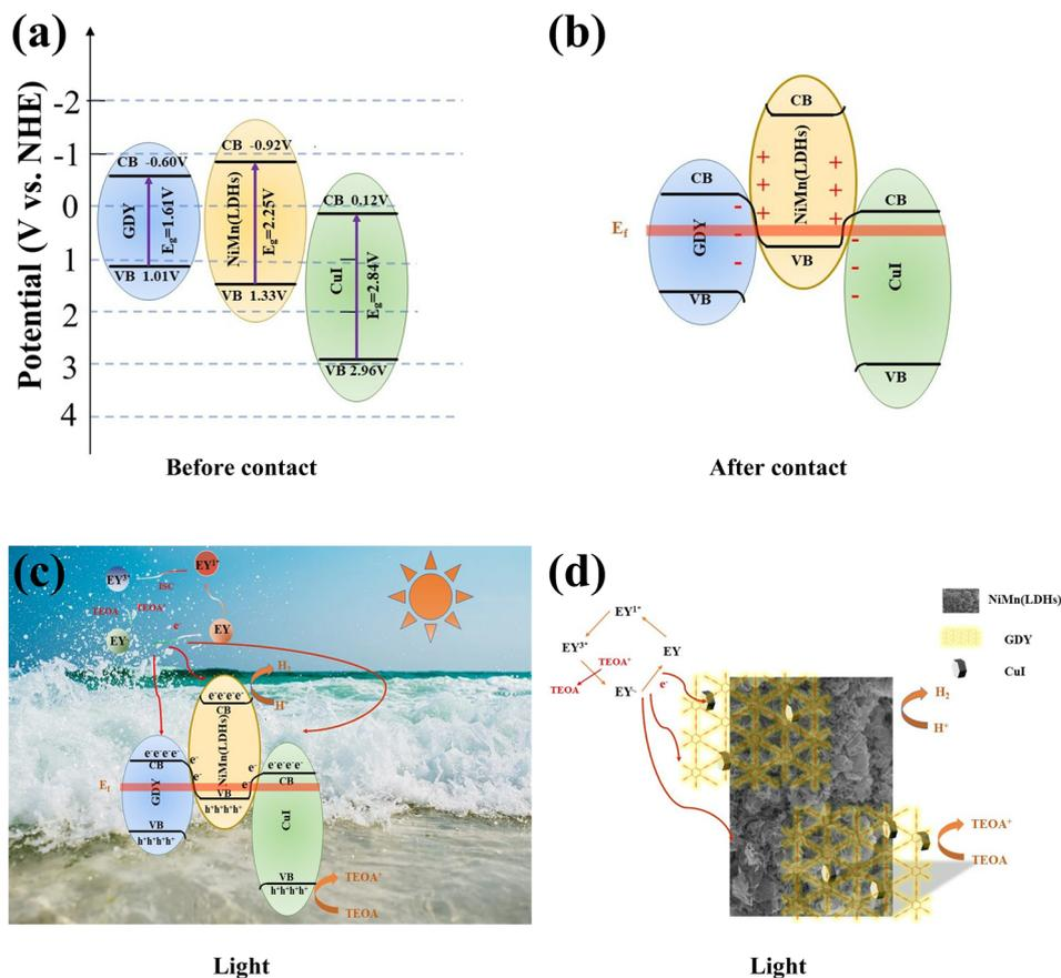
Fig. 11 (a and b) Double S-scheme heterojunction mechanism towards the charge transfer between CuI, GDY and NiMn(LDHs) before contact and after contact in darkness and under illumination. (c and d) Possible hydrogen evolution mechanism diagram for the GDY/CuI/NiMn(LDHs) photocatalyst.
