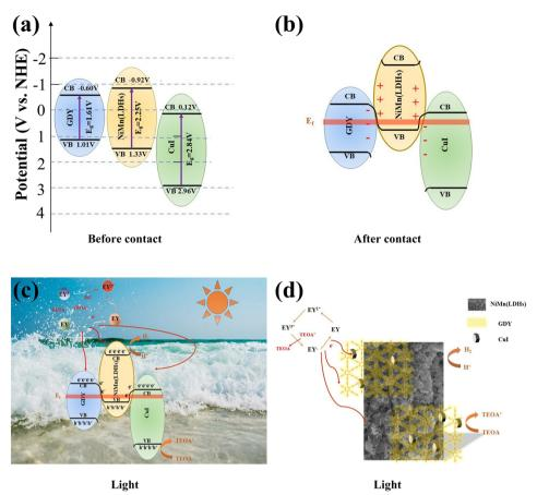
Fig. 11 (a and b) Double S-scheme heterojunction mechanism towards the charge transfer between Cul, GDY and NiMn(LDHs) before contact and after contact in darkness and under illumination. (c and d) Possible hydrogen evolution mechanism diagram for the GDY/Cul/NiMn(LDHs) photocatalyst.
