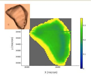
Fig. 4 The optical image of the carriers with the overlap of the chemical infrared image generated by the ratio of the integration in the specific region of amide I and amide II bands (~1710-1480 cm<sup>-1</sup>) and the band identifying the glass carrier ( $\sim$ 1500–1300 cm<sup>-1</sup>). The colour scale bar ranges from higher biocatalyst concentrations (yellow areas) to not-detectable concentrations (blue areas).
