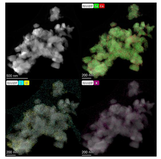
Fig. 2 HAADF-STEM images and corresponding compositional elemental mapping of the spent Fe<sub>9</sub>CoK<sub>6</sub> catalyst after 45 h time on stream at 300  $^{\circ}$ C with a H<sub>2</sub> to CO<sub>2</sub> ratio of 2 and a GHSV of 7200 mL  $g_{cat}$ <sup>-1</sup>  $h^{-1}$ .
