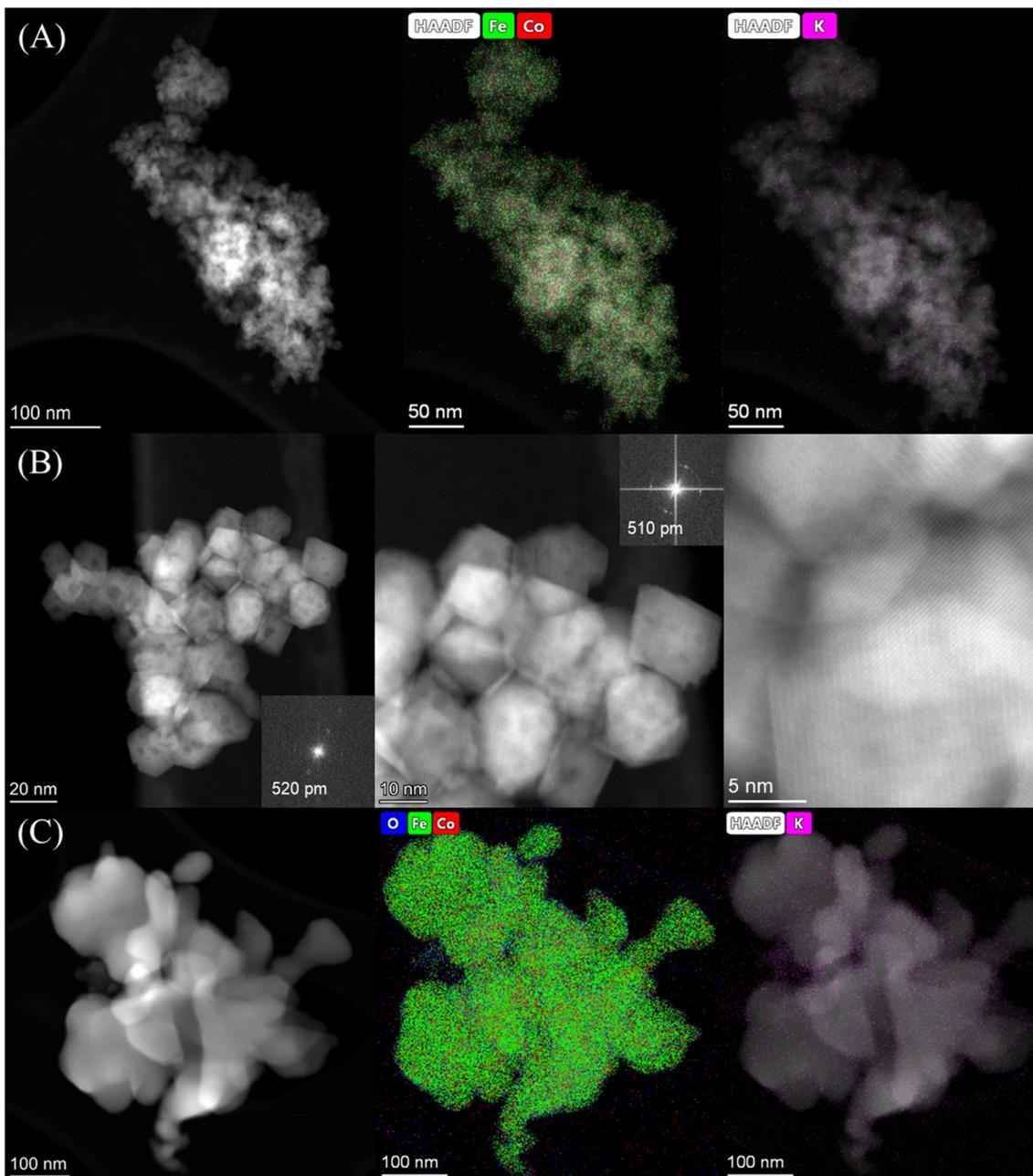
Fig. 1 HAADF-STEM images and corresponding elemental mapping images of the Fe<sub>9</sub>Co<sub>6</sub> catalyst (A and B) before reduction and (C) after reduction. The insets in B show the FFT patterns.
