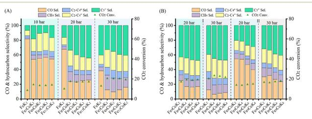
Fig. 4 Catalytic performance of Fe-Co catalysts under different pressures at 250 °C with a  $H_2$  to CO<sub>2</sub> ratio of 2 and GHSVs of 3600 mL  $g_{cat}^{-1}$  h<sup>-1</sup> (A and B-zone I) and 7200 mL  $g_{cat.}^{-1} h^{-1}$  (B-zone II).
