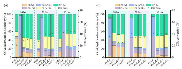
Fig. 5 Catalytic performance of Fe<sub>9</sub>CoK catalysts with different K loadings under different pressures at 300 °C with a H<sub>2</sub> to CO<sub>2</sub> ratio of 2 and GHSVs of (A) 3600 mL  $g_{cat.}^{-1} h^{-1}$  and (B) 7200 mL  $g_{cat.}^{-1} h^{-1}$ .
