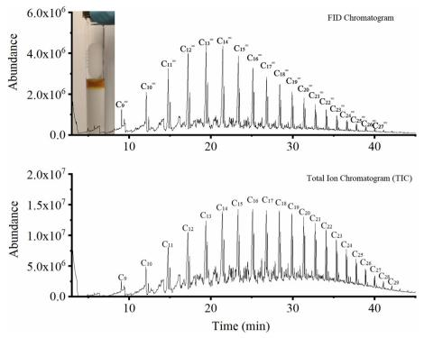
Fig. 7 GC-MS FID and total iron chromatogram of the liquid products.
