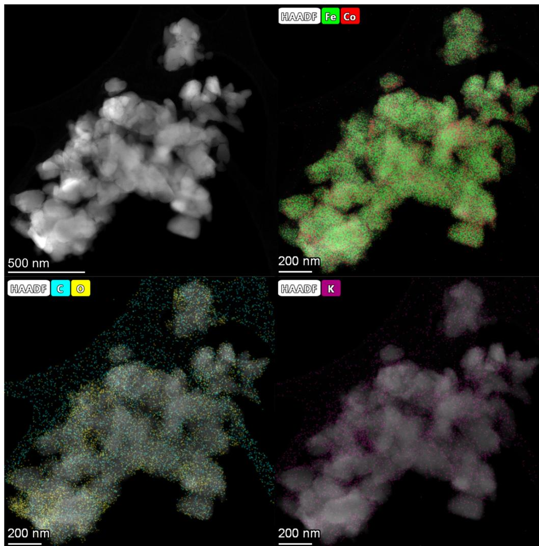
Fig. 2 HAADF-STEM images and corresponding compositional elemental mapping of the spent  $\text{Fe}_9\text{CoK}_6$  catalyst after 45 h time on stream at 300 °C with a  $\text{H}_2$  to  $\text{CO}_2$  ratio of 2 and a GHSV of 7200  $\text{mL g}_{\text{cat}}^{-1} \text{h}^{-1}$ .
