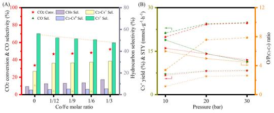
Fig. 6 (A) Catalytic performance of FeCoK catalysts with varying Co/Fe ratios at 20 bar; (B) C<sub>5</sub><sup>+</sup> yield (ball) and C<sub>5</sub><sup>+</sup> STY (star) together with O/P (C2-C4) ratios (triangle) for the FeK2 (orange), Fe3CoK2 (olive) and Fe9CoK2 (red) catalysts at different pressures. Other reaction conditions: 300 °C at a  $H_2$  to  $CO_2$  ratio of 3 and a GHSV of 3600 mL  $g_{cat.}^{-1} h^{-1}$ .
