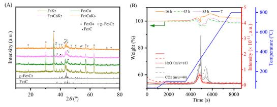
Fig. 3 (A) XRD patterns of the spent catalysts with 16 h TOS and (B) TGA-MS profiles of the spent Fe<sub>9</sub>CoK<sub>6</sub> catalysts with different TOS at 300 °C with a  $H_2$  to  $CO_2$  ratio of 2 and GHSVs of (A) 3600 mL  $g_{cat}$ .  $^{-1}$   $h^{-1}$  and (B) 7200 mL  $g_{cat}$ .  $^{-1}$   $h^{-1}$ .
