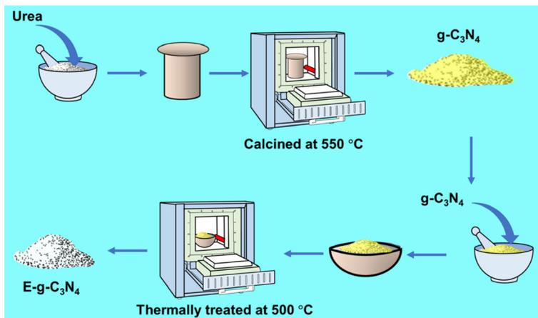
Scheme 1 Schematic presentation for the synthesis of  $g-C_3N_4$  and E- $g-C_3N_4$ .
