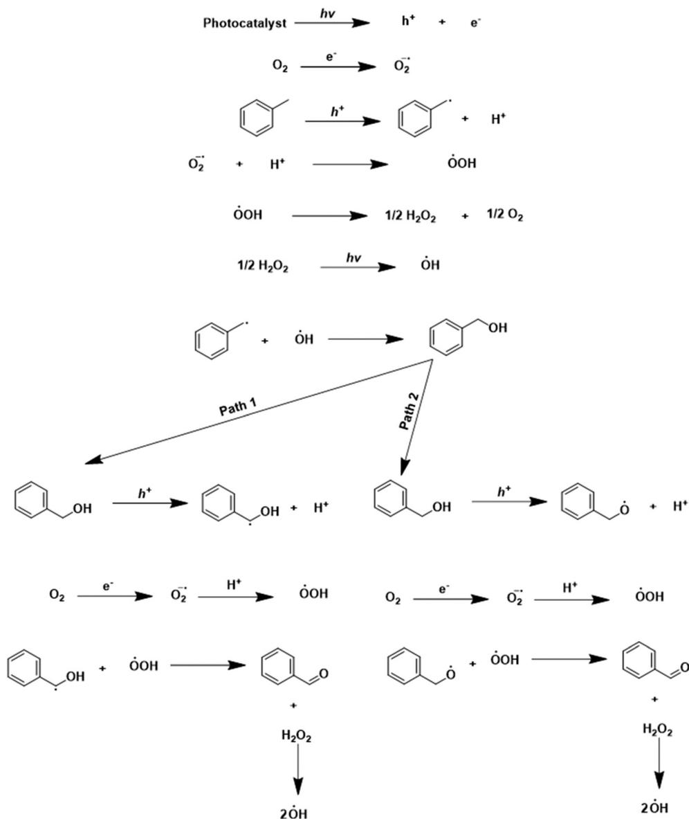
**Scheme 2** Possible mechanism and reaction steps associated with photocatalytic toluene oxidation.
