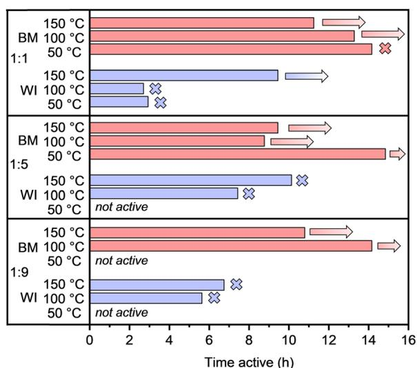
Fig. 3 Activity time (above 95% conversion of acetylene) of PdAg ( $x:y = 1:1; 1:5; 1:9$ ) catalysts supported on  $\alpha\text{-Al}_2\text{O}_3$  prepared by wet impregnation (WI, LSA) and ball milling (BM, HSA) at 50, 100, and 150 °C (reactor temperature). Crosses mark catalysts for which deactivation was observed; arrows are assigned to catalysts for which no sign of deactivation (conversion drop below 95%) was observed before the reaction was interrupted.
