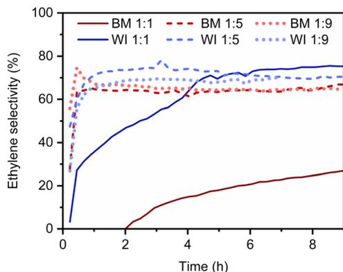
Fig. 2 Selectivity towards ethylene formation vs. time on stream for 1 wt% PdAg ( $x:y = 1:1; 1:5; 1:9$ ) catalysts supported on  $\alpha\text{-Al}_2\text{O}_3$  prepared by wet impregnation (WI, LSA) and ball milling (BM, HSA) at 150 °C (reactor temperature).
