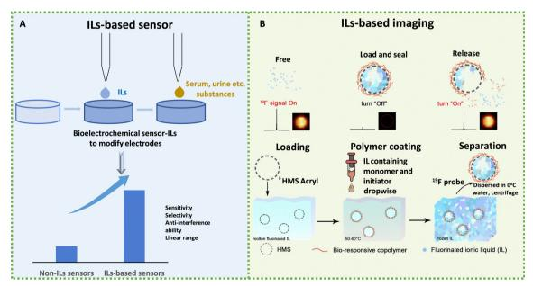
Fig. 7 Schematic diagram of the application of ILs in disease diagnosis. (A) Schematic diagram of IL-based sensors to test substances. (B) Schematic diagram of the <sup>19</sup>F MRI platform for stimuli-responsive <sup>19</sup>F MRI. Reproduced with permission from ref. 210. Copyright 2020 Elsevier.
