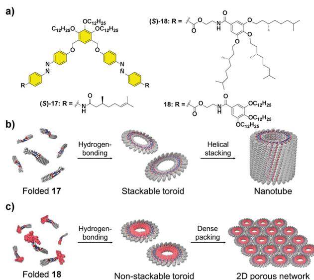
**Fig. 9** Molecular structures of scissor-shaped azobenzene dyads **17** and **18** (a) and illustrations of the self-assembly of **17** into nanotubes (b) and **18** into 2D porous networks (c) (reproduced from ref. 69 with permission from Wiley-VCH, copyright 2022).
