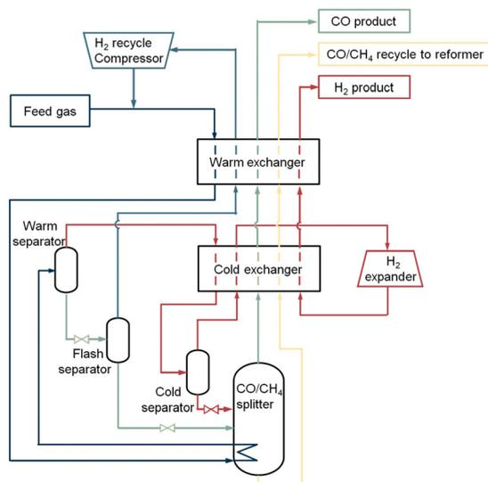
Fig. 4 Low-temperature partial condensation process. Figure based on process scheme from Dutta *et al.*<sup>31</sup>
