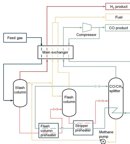
Fig. 5 The liquid methane wash process. Figure based on process scheme from Dutta *et al.*<sup>31</sup>
