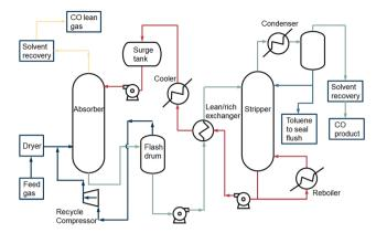
The basic COSORB process. Figure based on process scheme presented in Keller et al. 38
