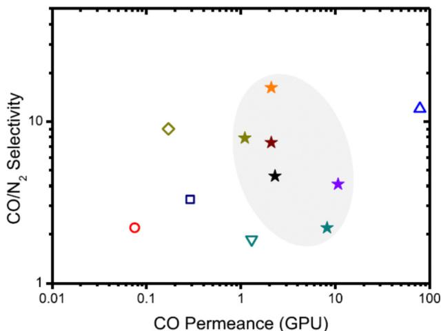
Fig. 12 Plot of CO/N<sub>2</sub> selectivity versus CO permeance for various membranes. Star symbols (\*) represent ref. 155. The blue triangle represents ref. 156, the other symbols represent ref. 151, 152, 158 and 159. Reprinted from ref. 155, Copyright (2021) with permission from Elsevier.
