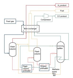
Fig. 5 The liquid methane wash process. Figure based on process scheme from Dutta et  $aL^{31}$
