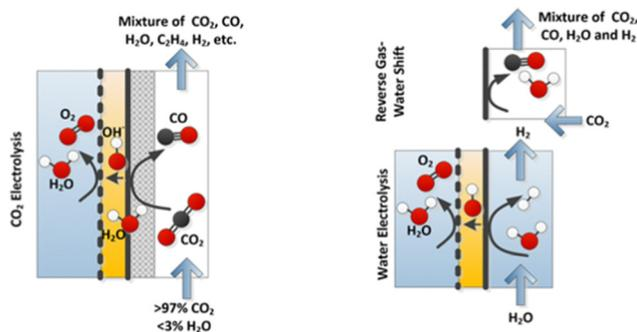
Fig. 14 Direct CO<sub>2</sub> to CO conversion (left), in this case in a reactor with a liquid anode (zero-gap) and CO<sub>2</sub> reduction at the vapour-fed cathode, and indirect CO<sub>2</sub> conversion (right), *via* water electrolysis and Reverse Gas–Water Shift Reaction (RGWSR). For simplicity, reaction stoichiometry is ignored.
