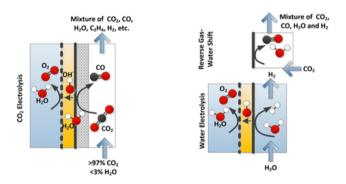
Fig. 14 Direct CO<sub>2</sub> to CO conversion (left), in this case in a reactor with a liquid anode (zero-gap) and CO2 reduction at the vapour-fed cathode, and indirect CO2 conversion (right), via water electrolysis and Reverse Gas-Water Shift Reaction (RGWSR). For simplicity, reaction stoichiometry is
