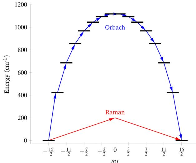
Fig. 1 Two main mechanisms of magnetic relaxation arising from spin-phonon coupling in single-molecule magnets, Orbach (blue) and Raman (red), illustrated for the  $J = 15/2$  multiplet of a  $\text{Dy}^{3+}$  SMM with a strong uniaxial crystal field.
