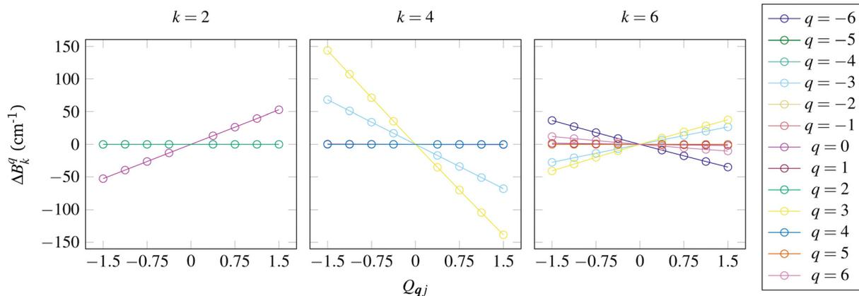
Fig. 7 Change in each  $B_k^q$  from the equilibrium values for [Yb(trens)] as a function of mass- and frequency-weighted dimensionless displacement  $Q_{qj}$  along a vibrational mode.<sup>42</sup> Note that this mode is a totally-symmetric vibrational mode so that the  $C_3$  symmetry of [Yb(trens)] is not broken and hence only certain  $B_k^q$  are affected; hence, some are overlapping with zero magnitude.
