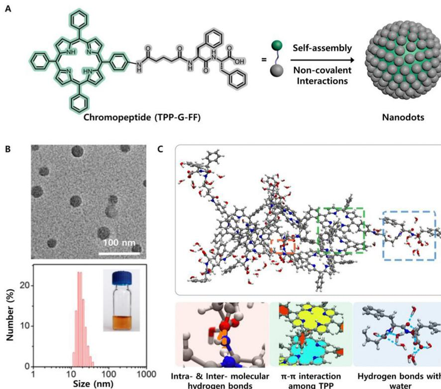
Fig. 5 (A) Schematic illustration of the self-assembly of a peptide–porphyrin conjugate (TPP-G-FF) into photothermal nanodots. (B) TEM image and DLS size distribution of the nanodots. The inset shows a picture of the nanodots in an aqueous solution. (C) Underlying intermolecular interaction mechanism of TPP-G-FF molecules obtained by MD simulation. Reproduced from ref. 53 with permission from the American Chemical Society, copyright [2017].
