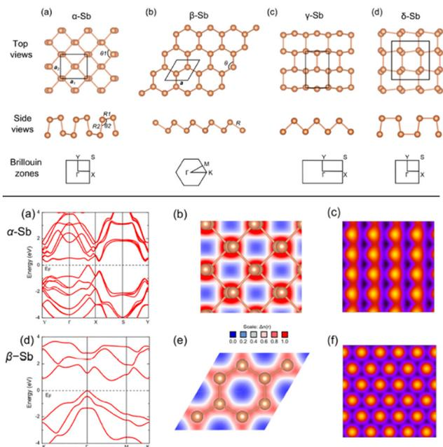
**Fig. 6** Top: Structural configurations of antimonene allotropes: (a)  $\alpha$ -Sb, (b)  $\beta$ -Sb, (c)  $\gamma$ -Sb, and (d)  $\delta$ -Sb. Bottom: Electronic properties of (a)–(c)  $\alpha$ -Sb and (d)–(f)  $\beta$ -Sb monolayers: (a), (d) band structure, (b), (e) charge density projected in the plane, and (c), (f) simulated scanning tunneling microscopy (STM) images. Adapted from ref. 35 with permission from American Chemical Society, copyright 2015.
