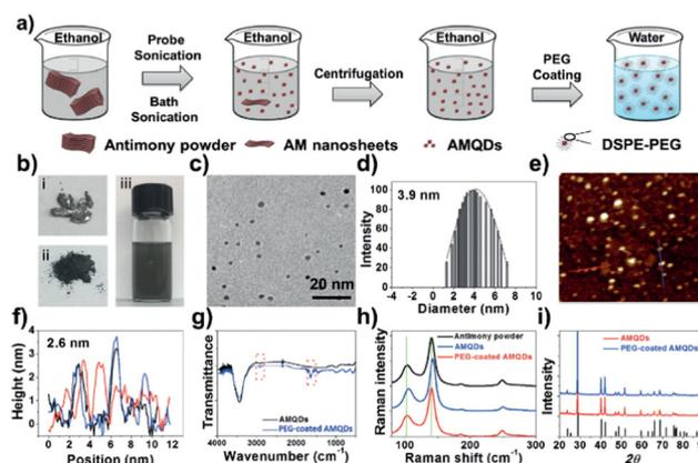
**Fig. 12** (a) Fabrication of PEG-coated AMQDs. (b) Images of bulk antimony, antimony powder, and AMQD solution during the preparation process. (c) TEM image, (d) diameter distribution, (e) AFM image, and (f) thickness of the PEG-coated AMQDs. (g) FTIR spectrum, (h) Raman spectrum, and (i) XRD spectrum of AMQDs and PEG-coated AMQDs. Reproduced from ref. 127 with permission from John Wiley & Sons, copyright 2017.
