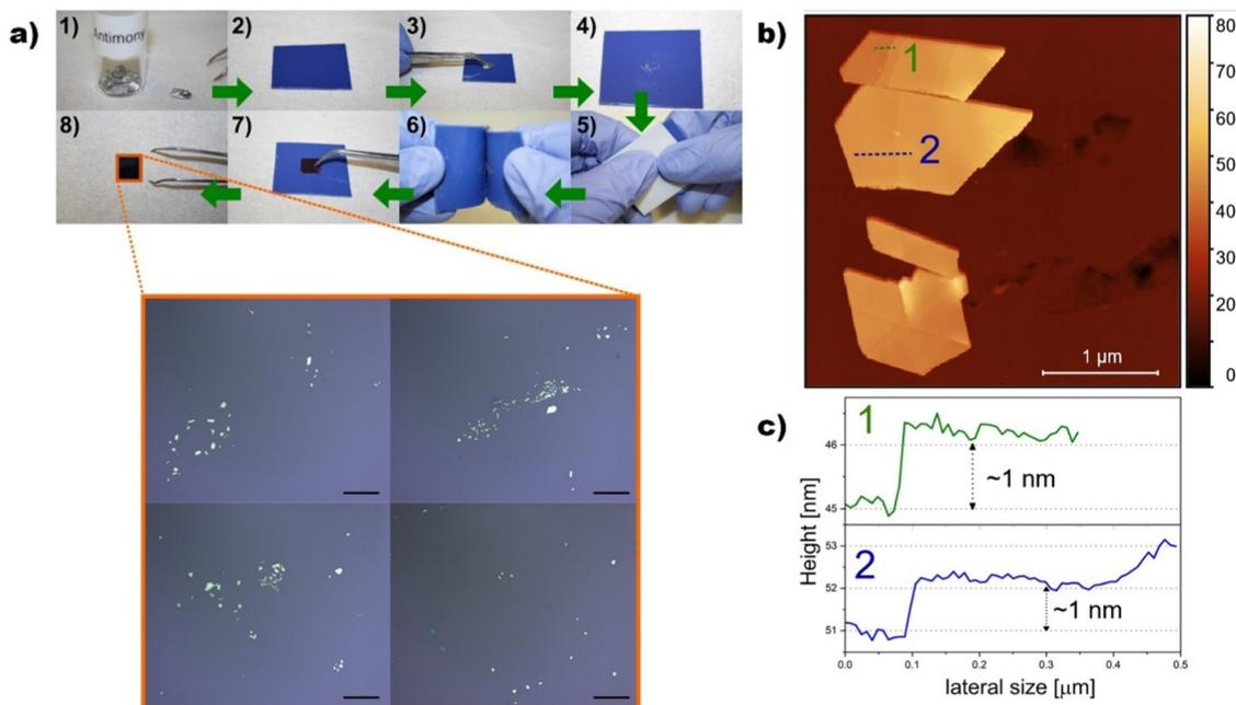
**Fig. 7** (a) Step-by-step procedure (1–8) for the exfoliation of ANSs using micromechanical approach. Inset in (8) Optical micrographs showing exfoliated ANSs with different polygonal geometries. Scale bars 20  $\mu$ m. (b) AFM image of typical ANSs and (c) height profiles along the dashed lines showing steps of approximately 1 nm, compatible with a single layer antimonene. Adapted from ref. 98 with permission from IOP Publishing, copyright 2020.
