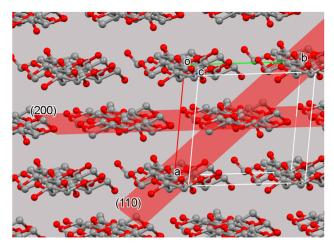
Fig. 2 The cellulose Iβ unit cell and surrounding molecules with the crystal (200) and (110) planes. The planes extend the entire dimensions of the crystal and are found for each unit cell. The chemically repeated unit of cellulose is the glucose residue. In neat cellulose crystals the two-fold (or pseudo-two-fold) symmetry results in a crystallographic repeat distance that includes two glucose residues. Other cellulose structures have different repeat distances.12
