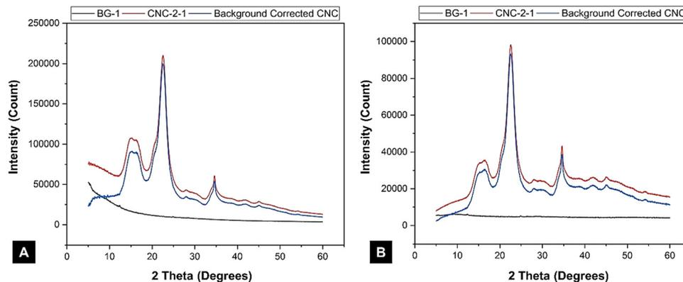
Fig. 7 Effect of the (A) fixed slit and (B) variable slit X-ray diffractometer on the background curve and the resulting corrected intensity of a cellulose nanocrystal (CNC) sample. Rietveld analysis software typically assumes a fixed-slit diffractometer configuration. These fixed-slit data were converted from variable-slit data with the Malvern-Panalytical HighScore software.
