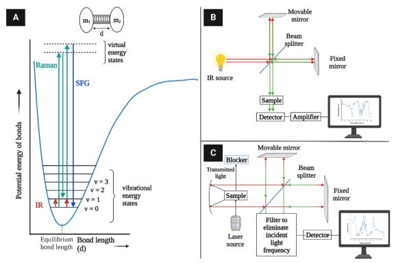
Fig. 10 (A) Vibration energy states of diatomic molecules and electronic transitions involved in IR absorption and Raman scattering. The diatomic molecules can be modeled as two masses ( $m_1$  and  $m_2$ ) connected with a spring constant  $k^{117}$  (redrawn from ref. 117). (B) A simplified schematic of typical IR instrumentation. (C) A Raman spectrometer setup
