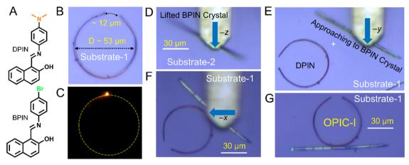
Fig. 37 (A) Molecular structures of DPIN and BPIN. Confocal micrographs portraying AFM-based, (B and C) mechanically bent truncated circular DPIN crystal, (D) mechanical lifting, (E and F) transferring and (G) moving (with positioning) to integrate a straight BPIN crystal with a truncated circular DPIN crystal to create μ-OPIC-I. Adapted with permission from ref. 438 Copyright 2020, Wiley-VCH.
