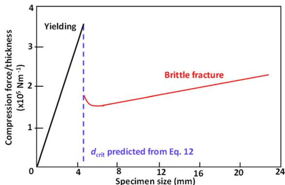
Fig. 44 Normalized force required to cause the brittle fracture of a large particle (red line) or yield of a small particle (black line) of polystyrene. The vertical dashed line signifies the value of  $d_{crit}$  predicted from eqn (12). Adapted with permission from ref. 477 Copyright 1978, Nature Publishing Group.
