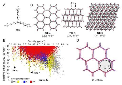
Fig. 23 Comparison of the predicted and experimental structures and properties for molecule T2E whose molecular structure is shown in panel (A). The predicted crystal energy landscape for T2E is shown in panel (B). Selected structures for T2E from the energy-density landscape are shown in panel (C). An overlay of the predicted (red) and experimental (blue) structures for T2E is given in panel (D). Adapted with permission from ref. 326 Copyright 2017, Springer Nature.
