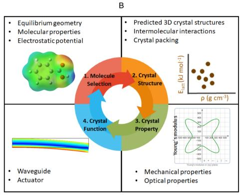
Fig. 21 (a) Most commonly used computational methods for predicting the mechanical properties and effects of crystalline materials. The arrow at the bottom shows the length scale on which each modelling technique applies. DFT = density functional theory, MD = molecular dynamics, and FEM = finite element methods. (b) Proposed steps in the in silico discovery of mechanically responsive molecular crystals
