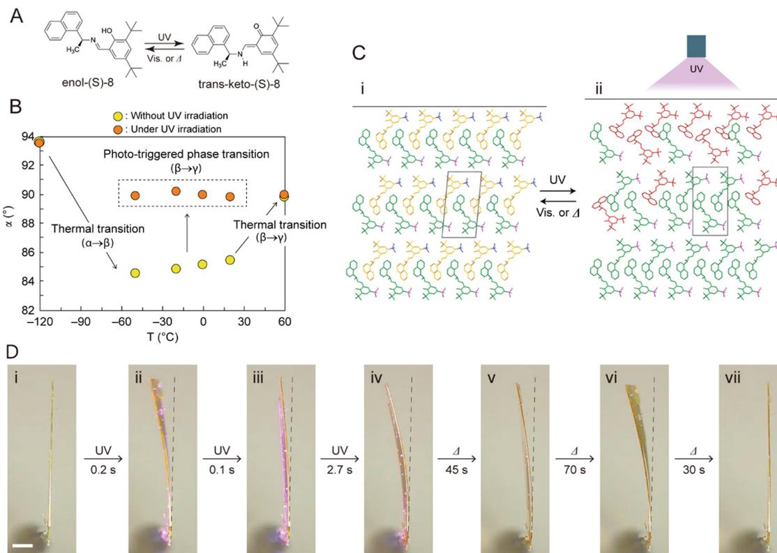
Fig. 41 (A) Enol–keto photoisomerization of a chiral salicylideneamine, (S)-**8**. (B) Phototriggered phase transition based on the change of angle  $\alpha$ . (C) Mechanism of the phototriggered phase transition. (D) Stepwise bending of a thin plate-like crystal of enol-(S)-**8** upon UV irradiation. Scale bar, 500  $\mu\text{m}$ .<sup>462</sup> Adapted with permission from ref. 462 Copyright 2019, Springer Nature.
