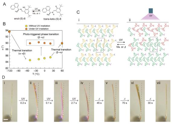
Fig. 41 (A) Enol-keto photoisomerization of a chiral salicylideneamine, (S)-8. (B) Phototriggered phase transition based on the change of angle α. (C) Mechanism of the phototriggered phase transition. (D) Stepwise bending of a thin plate-like crystal of enol-(S)-8 upon UV irradiation. Scale bar, 500 μm. 462 Adapted with permission from ref. 462 Copyright 2019, Springer Nature.
