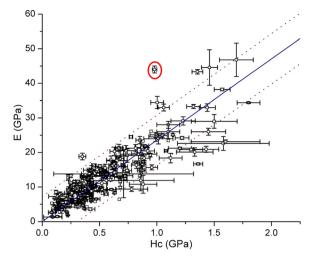
Fig. 43 Elastic modulus (E) and indentation hardness ( $H_c$ ) of molecular crystals vary over a wide range. Adapted from ref. 27. Copyright 2020, The Royal Society of Chemistry.
