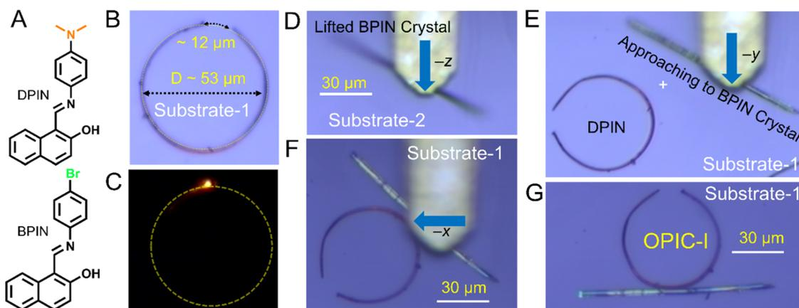
Fig. 37 (A) Molecular structures of **DPIN** and **BPIN**. Confocal micrographs portraying AFM-based, (B and C) mechanically bent truncated circular **DPIN** crystal, (D) mechanical lifting, (E and F) transferring and (G) moving (with positioning) to integrate a straight **BPIN** crystal with a truncated circular **DPIN** crystal to create  $\mu$ -OPIC-I. Adapted with permission from ref. 438 Copyright 2020, Wiley-VCH.
