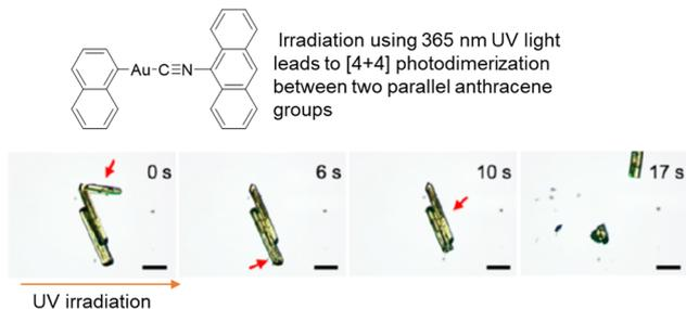
**Fig. 10** Optical micrographs of microcrystals of an aryl(9-isocyananthracene)gold(i) complex exhibiting photosalient effects when irradiated with UV light (365 nm). The thick red arrows indicate the position of the crystals that jumped. Scale bars represent 50  $\mu\text{m}$ .<sup>218</sup> Adapted with permission from ref. 218 Copyright 2021, American Chemical Society.
