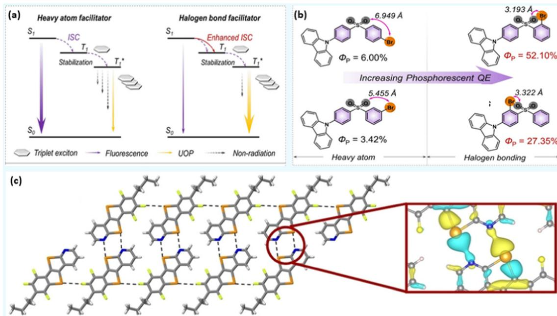
Fig. 4 (a) Proposed mechanisms for heavy atom and halogen bonding facilitated ISC in ultralong organic phosphors, and (b) phosphorescence enhancement *via* XB in **10–13** (UOP = ultralong organic phosphorescence). (c) X-ray stick representation of the supramolecular nanoribbon developed by **20a**. Local charge density is zoomed. Reproduced with permission from ref. 1 (Copyright (2020) Wiley-VCH GmbH) and ref. 53 (Copyright (2022) The Authors. *Angewandte Chemie* published by Wiley-VCH GmbH).
