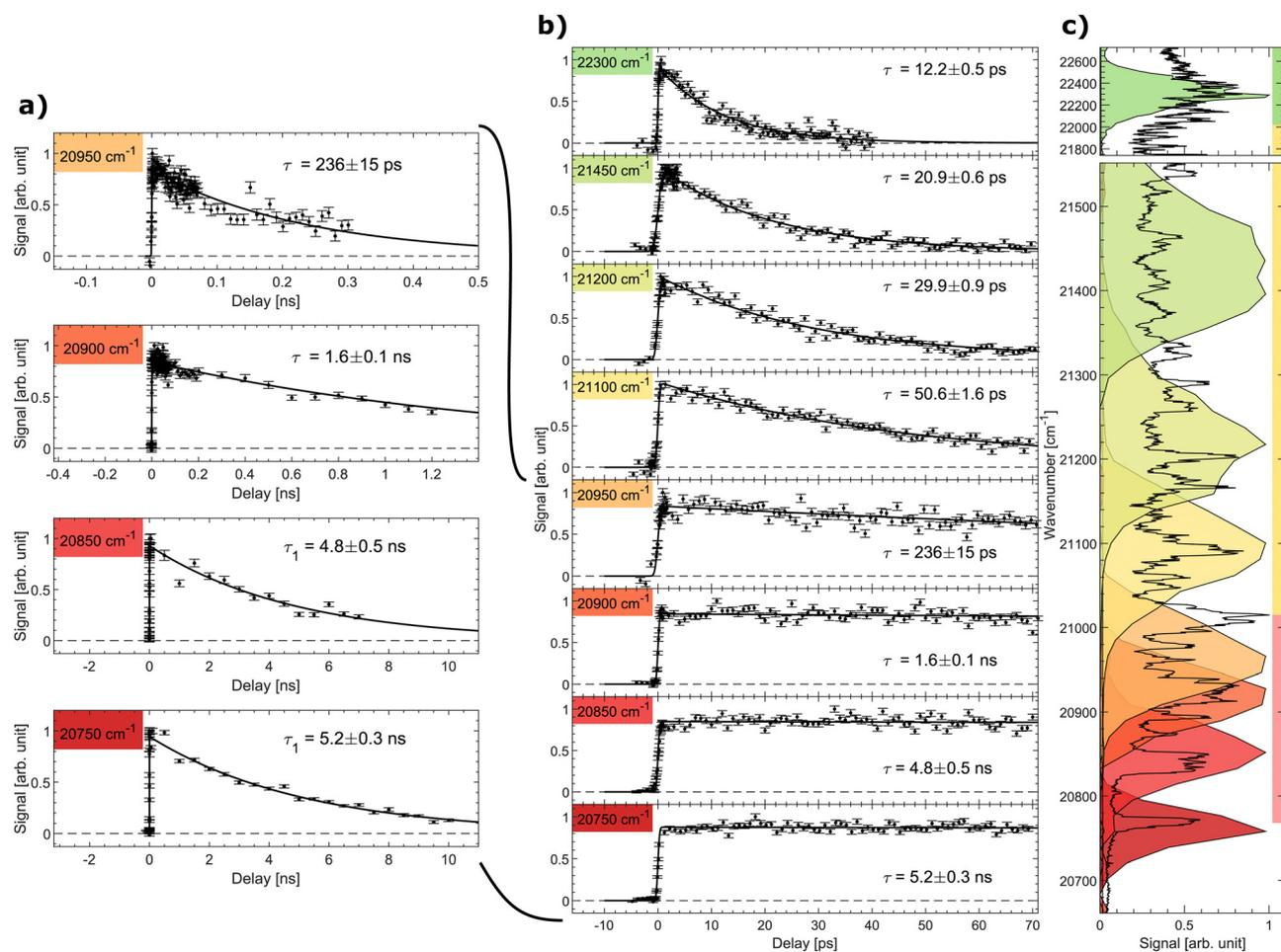
Fig. 3 Signal as a function of pump-probe delay recorded at different photon energies (given in  $\text{cm}^{-1}$ ). (a) Decays with long ns lifetimes, (b) all data (pump-probe delays up to 70 ps). (c) The recorded pulse shape of the pump pulses are shown as colored areas overlaid on the vibrationally resolved prompt action-absorption spectrum of  $\text{HBDI}^-$ .<sup>31</sup> See Fig. 2 for the color code applied on the vertical axis of panel (c).
