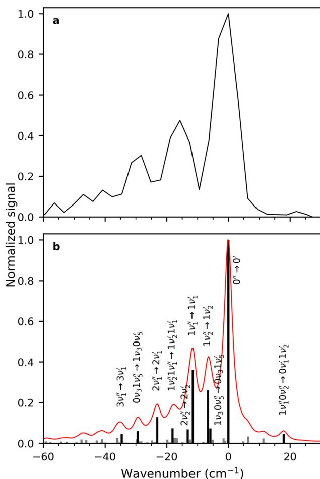
Fig. 4 (a) Zoom in on the main absorption band in the fluorescence-excitation spectrum of  $\mathbf{R}^-$ . The energy separations between the peaks are approximately  $15\text{ cm}^{-1}$ . (b) Simulated absorption spectrum of  $\mathbf{R}^-$  at a temperature of  $100\text{ K}$  (red) from the transitions shown in grey (no labels) and black. The vibrational quantum number is followed by the name of the mode and '' refers to  $S_0$  and ' to  $S_1$ .
