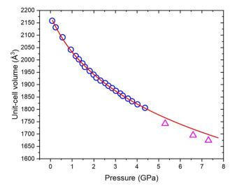
Fig. 7 Variation of unit-cell volume as a function of pressure for Form I (open blue circles) obtained from neutron powder diffraction data; the EoS fit from P-V data (solid red line); and unit-cell volumes for Form II obtained from single crystal X-ray diffraction data.
