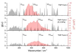
**Fig. 9** Vibrational  $q(\omega)$  plots (grey) for Form I at ambient pressure. Form I re-optimised at 5.3 GPa, and Form II at 5.3 GPa, alongside their corresponding  $\Omega^{(2)}$  envelopes (red).
