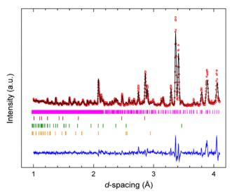
Fig. 2 Rietveld refinement of neutron powder diffraction pattern of 3,4,5-TNP at 0.08(3) GPa (space group P2<sub>1</sub>/c); red dots are experimental (observed) data, solid black line is the calculated profile from the refinements, while the bottom blue line shows the residual intensities I(obs)-I(calc). Simulated Bragg reflections for each phase are shown as vertical tick marks: from top to bottom 3,4,5-TNP, Pb (the pressure calibrant),  $Al_2O_3$ , and  $ZrO_2$  (the anvil material).
