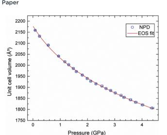
Fig. 3 Variation of unit-cell volume as a function of pressure determined from neutron powder diffraction data for 3,4,5-TNP (open blue circles) and the EoS fit from P-V data (solid red line). Error bars are shown, but are smaller than the symbols.
