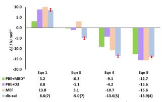
Fig. 2 Cocrystal interconversion energies (in kJ mol<sup>-1</sup>) obtained from periodic DFT calculations, molecular energy frameworks (MEF) and dissolution calorimetry (dis-cal) measurements. Red error bars are shown for the energies measured by dis-cal.
