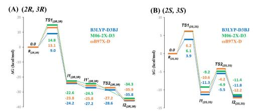
Fig. 3 Free energy profile for the enzyme-substrate complexes with the substrate poses that would lead to the (A) (2R,3R) product or (B) (2S,3S) product. Geometry optimizations and frequency calculations were conducted using B3YLP-D3(BJ), M06-2X-D3 and ωB97X-D with the 6/31G\* basis set.
