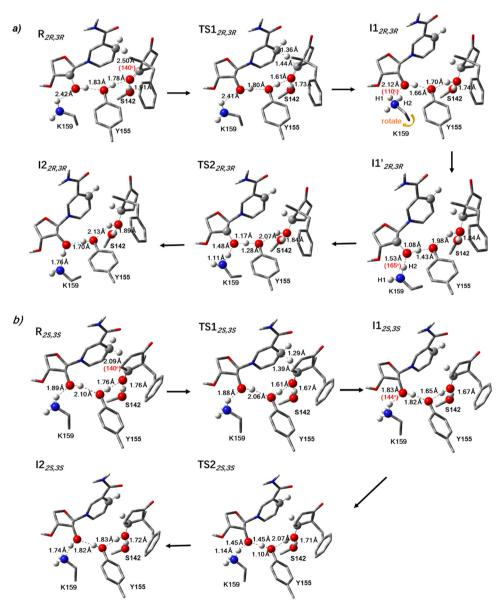
Fig. 5 Optimized geometries in the reaction pathways conducted using B3LYP-D3(BJ) with the 6/31G\* basis set. (a) Substrate pose leading to the dominant (2R,3R) product and (b) substrate pose that leads to the minor (2S,3S) product. (The number in parentheses in the reactant complex conformation is the bonding angle between the attacking hydrogen on C4 of NADPH and the carbonyl carbon of the substrate).
