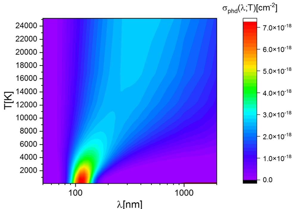
Fig. 3 The surface plot of average cross-section for photodissociation, against  $\lambda$  and  $T$ , of  $\text{H}_2^+$  molecular ion. The dataset is obtained in Srećković *et al.*<sup>45</sup>
