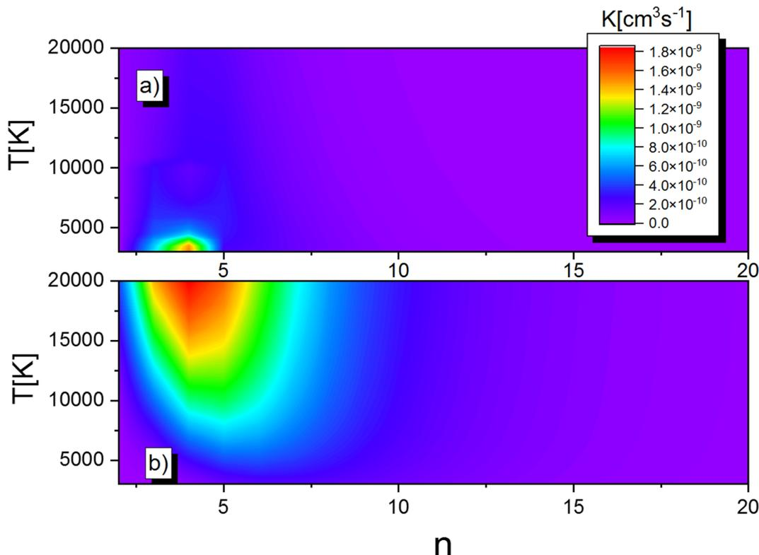
Fig. 4 (a) Rate coefficient for associative ionization channel (upper) of eqn (1) as a function of  $n$  and  $T$  for the case  $X = H$ . (b) same as a) but for non-associative ionization channel (lower) of eqn (1). Dataset is obtained in Srećković *et al.*<sup>54</sup>
