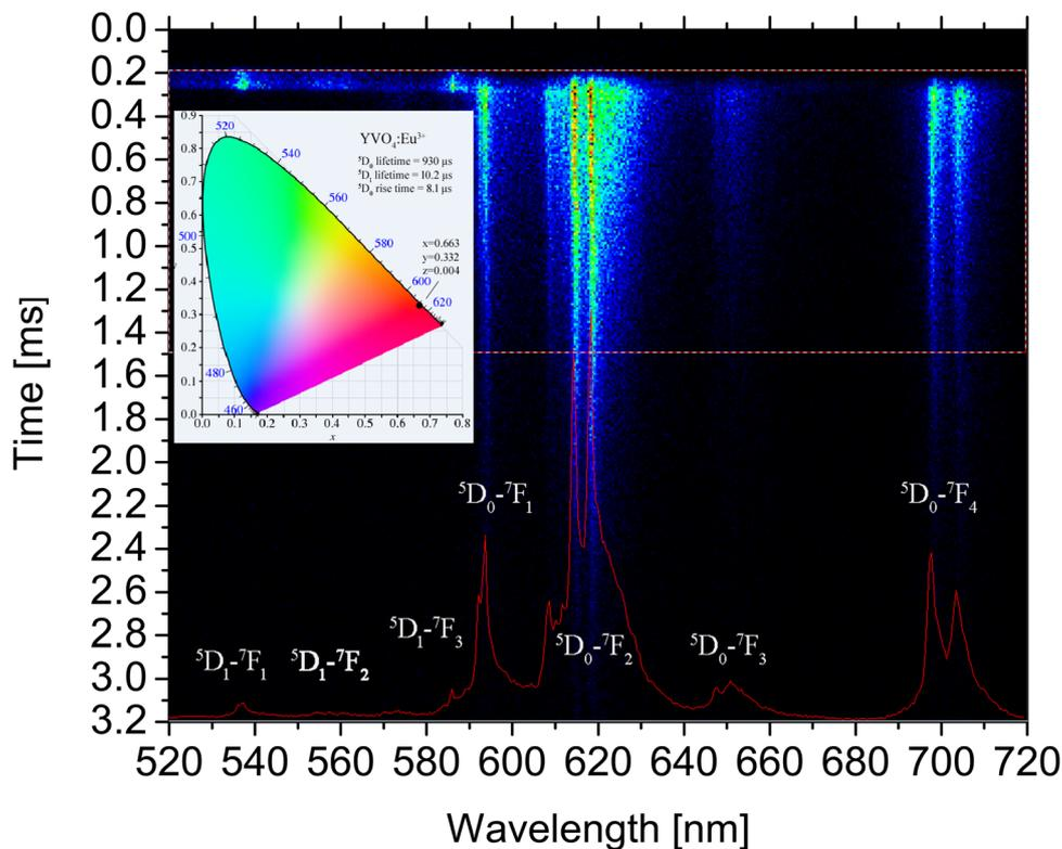
Fig. 6 Typical time-resolved spectrum of rare earth doped phosphor ( $\text{YVO}_4:\text{Eu}$ ) acquired in our measurements. Europium transitions are denoted. Inset shows CIE plot (color coordinate diagram) calculated from spectral data.
