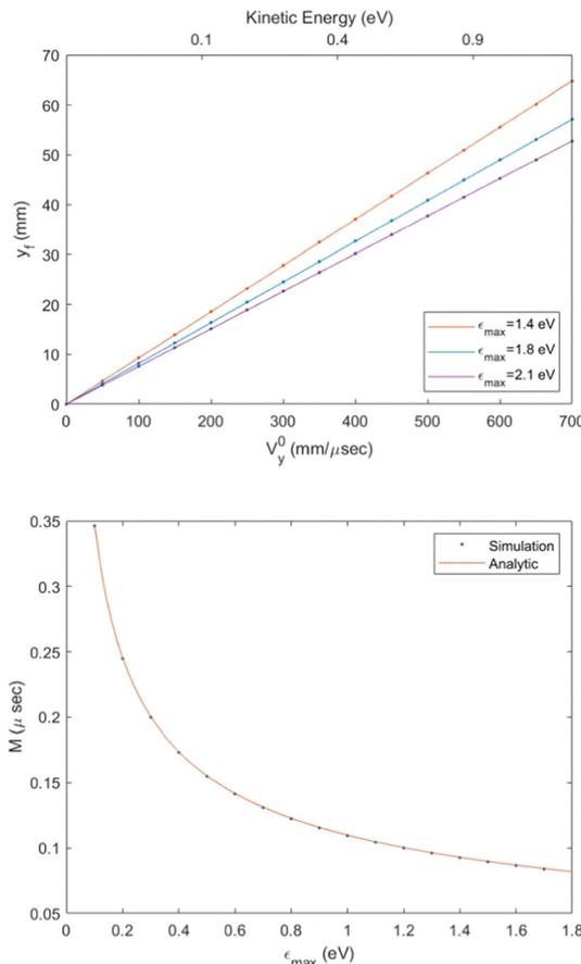
**Fig. 4** (a) The final position on the detector as a function of the initial velocity, for electrons that are starting from the origin with initial velocity on  $y$  axis only, for different values of  $\epsilon_{\text{max}}$ . The continuous lines are given by the analytical derivation and the dots are given by the simulation. (b) The magnification as a function of  $\epsilon_{\text{max}}$ .
