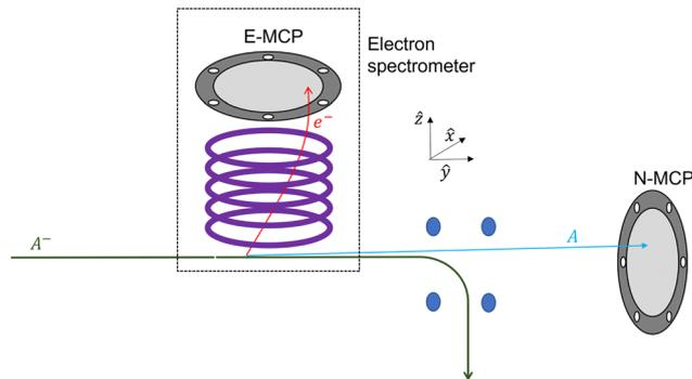
**Fig. 9** An illustration of a spectrometer for measuring the thermionic emission from anions without prior mass selection, as an example for an application of mixed imaging: velocity map imaging along the  $\hat{x}$  direction and position imaging in the  $\hat{y}$  direction which is used to determine the position of the ionization event. This information can be used to improve the time-of-flight determination of the parent ions mass.
