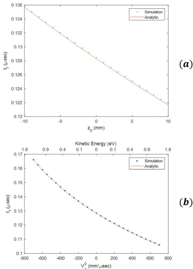
Fig. 5 (a) Time-of-flight for a beam of electrons starting from different positions along the  $\hat{z}$  axis between  $z_0 = -10$  mm to  $z_0 = 10$  mm, for  $x_0 = y_0 = 0$ , and for  $\epsilon_{\max} = 1.8$  eV. (b) Time-of-flight for a beam of electrons starting from the origin with velocity on  $z$  axis only for  $\epsilon_{\max} = 1.8$  eV.
