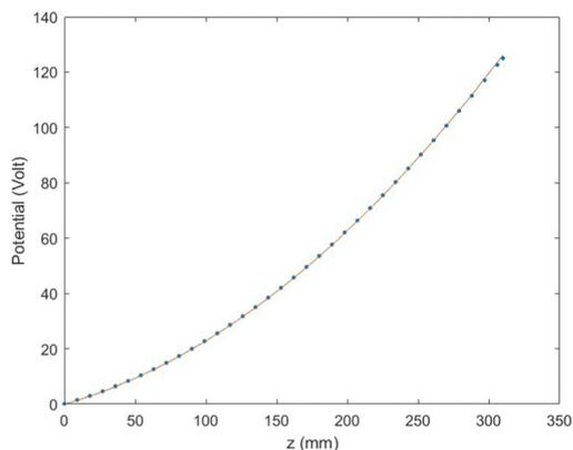
**Fig. 3** Comparison of the numerically calculated potential along the  $z$  axis (for the same value of  $\epsilon_{\text{max}}$  used in Fig. 2), as a function of  $z$ , to the analytical formula (eqn (2)). Here  $z = 0$  corresponds to the center of the interaction zone. We observe small deviations (up to 1.2%) from the analytical potential only at small distances ( $<15$  mm) from the detector.
