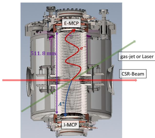
**Fig. 1** A schematic illustration of the CSR-ReMi. In this illustration the stored ion beam passes through the instrument from left to right (along the direction indicated by the red arrow), and is crossed by either a neutral gas jet or by laser (along the direction indicated by the green arrow). The resulting electrons are accelerated upwards and imaged on the E-MCP detector, while the resulting cationic fragments are accelerated in the opposite direction and imaged on the I-MCP detector.
