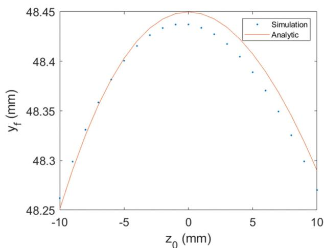
Fig. 6 Impact position  $y_f$  as a function of the source position  $z_0$ , for  $\epsilon_{\max} = 1.8$  eV. We used an electron beam starting from the origin with velocity on the  $y$  axis only, which corresponds to a kinetic energy of 1 eV. We observe very small deviations (less than 0.041%) that practically can be neglected, since they are smaller than the detector's resolution.
