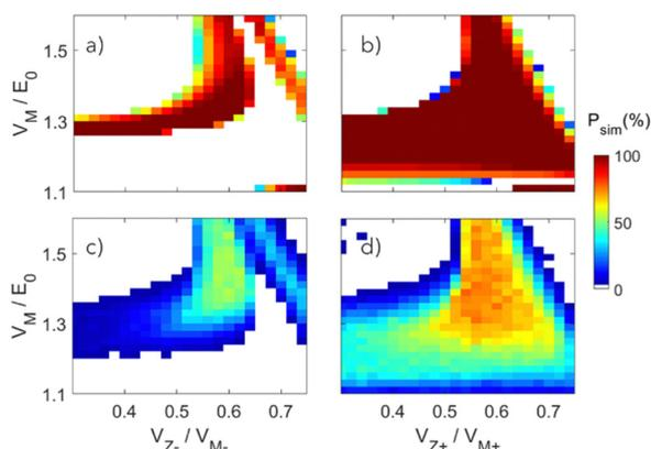
Fig. 7 Trapping efficiencies ( $P_{\text{sim}}$ ), simulated with the analytical HEIBT model. On the left (a) and (c) for the inner trap and on the right (b) and (d) for the outer HEIBT trap. Bottom panels (c) and (d) including and top panels (a) and (b) without ion–ion interaction.
