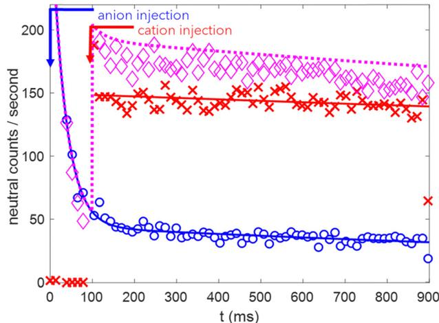
Fig. 3 Neutral CCD signal vs. trapping time for three sets of experiments. Blue for trapping of  $\sim 2.3$  keV  $SF_6^-$  ion beam in the inner HEIBT trap, red for a  $\sim 2.0$  keV  $SF_5^+$  ion beam in the outer trap and magenta diamonds for a merged beam experiment, in which both cations and anions produce neutral signal. The dotted magenta curve presents the sum of both single beam experiments (blue and red curves).
