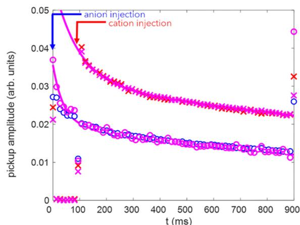
Fig. 5 Mass selective, time dependent pickup FFT detection of a merged beam experiment in the HEIBT. Blue for  $SF_6^-$  anions in the inner trap and red for  $SF_5^+$  cations in the outer HEIBT trap. Magenta for merged beam experiment while circles represents anions and crosses represent cations.
