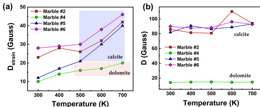
Fig. 5 Variations of (a)  $D_{\text{strain}}$  vs. temperature and (b) ZFS ( $D$ -tensor) vs. temperature, for marbles #2, #4, #5, and #6.
