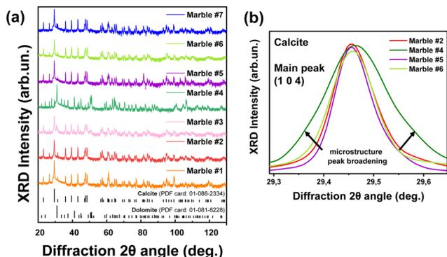
Fig. 7 (a) XRD patterns from collected Greek marbles and their major crystal phases, *i.e.* dolomite and calcite. (b) Magnified region of the main peak (1 0 4) of the Greek marbles, demonstrating the peak broadening as the microstrain increases.
