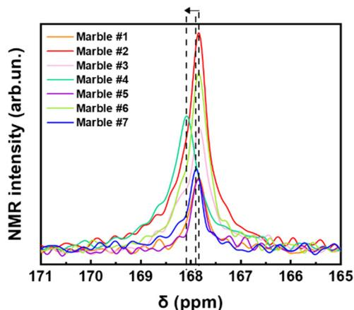
Fig. 6  $^{13}\text{C}$  NMR spectra of all marbles magnified in the carbonate's region.
