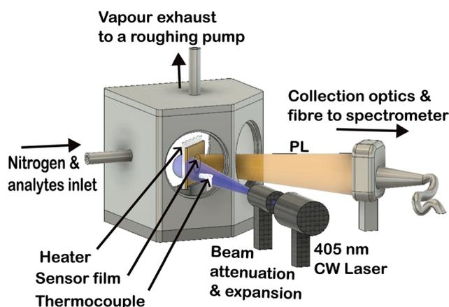
Fig. 1 Experimental setup for sensing and thermal release of explosives.
