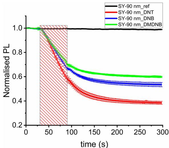
Fig. 3 SY response to nitroaromatic analytes (DNT and DNB) and a taggant (DMDMB); the normalised PL is obtained by integrating the PL intensity across the wavelengths and normalising. The rectangle strip bar indicates the duration of analytes exposure. Each quenching experiment was repeated three times, and the solid lines show the average.
