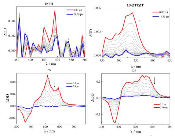
Fig. 2 Triplet transient absorption spectra obtained in nitrogen-purged Tol solutions of 1NPH, 2,5-(2TE)<sub>2</sub>T, PN and DF<sup>45</sup> ( $\lambda_{\text{exc}} = 355 \text{ nm}$ )
