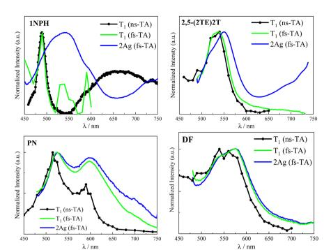
Fig. 6 Comparison between T<sub>1</sub> ESA spectra as obtained by ns-TA (black, scattered-line) and by fs-TA (green line) experiments and 2Ag ESA spectra as obtained by fs-TA experiments (blue) for compounds **1NPH**, **2,5-(2TE)**<sub>2</sub>**T**, **PN** and **DF** in Tol.
