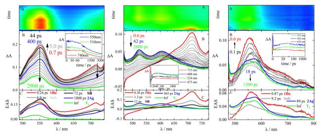
Fig. 3 Fs-TA measurements of compounds 2,5-(2TE)<sub>2</sub>T (left), PN (central) and DF (right) in Tol ( $\lambda_{pump} = 400 \text{ nm}$ ). Panel A: experimental 3D matrix; Panel B: representative spectra at different delay times and representative kinetics (inset) at different wavelengths; and Panel C: EAS (evolution associated spectra) obtained by global analysis.
