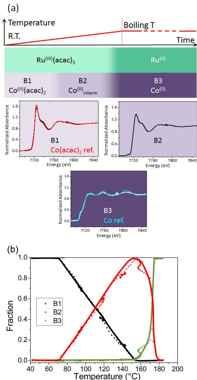
Fig. 7 (a) Spectra at the Co K-edge of the species B1, B2 and B3 extracted with the MCR-ALS method during heating a solution of  $\text{Co}(\text{acac})_2$  and  $\text{Ru}(\text{acac})_3$  in octan-1-ol for the  $\text{Co}_{80}\text{Ru}_{20}$  composition. Spectra at the Co K-edge of the  $\text{Co}(\text{acac})_2$  and Co references are also given for comparison purposes. (b) Speciation diagram for the B1, B2 and B3 species as a function of temperature, tendency extracted from Fig. S20 (ESI†).
