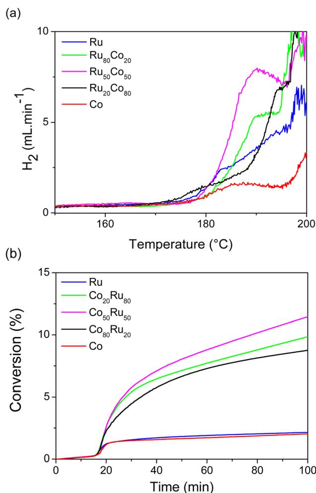
Fig. 8 (a) Instantaneous  $\text{H}_2$  flow measured during the synthesis of the  $\text{Co}_x\text{Ru}_{100-x}$  NPs and (b) calculated octan-1-ol conversion using the total volume of evolved  $\text{H}_2$ .
