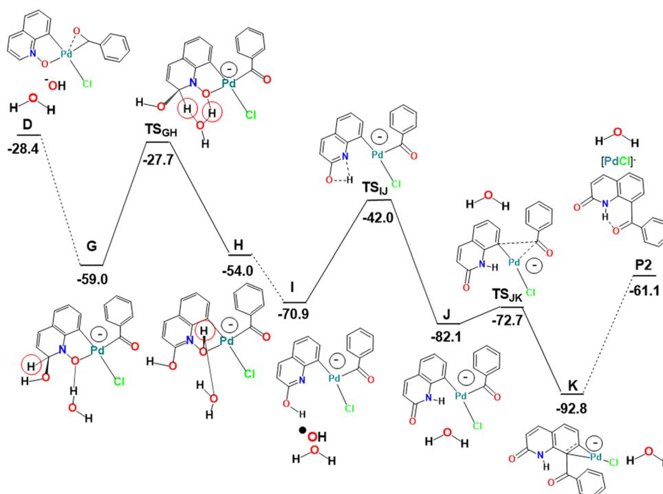
Fig. 3 Energy profile for the second part of the alternative functionalization at C8 and functionalization at C2 of QO in the presence of water (relative Gibbs energies in kcal mol<sup>-1</sup> in dichloroethane; the negative charge represents the charge of the complex and the red circle highlights the hydrogen migrating in the G to H transformation).
