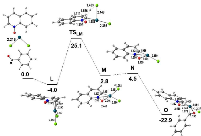
Fig. 5 Energy profile for the first part of the functionalization of QO at C2 (relative Gibbs energies in kcal mol<sup>-1</sup> in dichloroethane; distances in Å).
