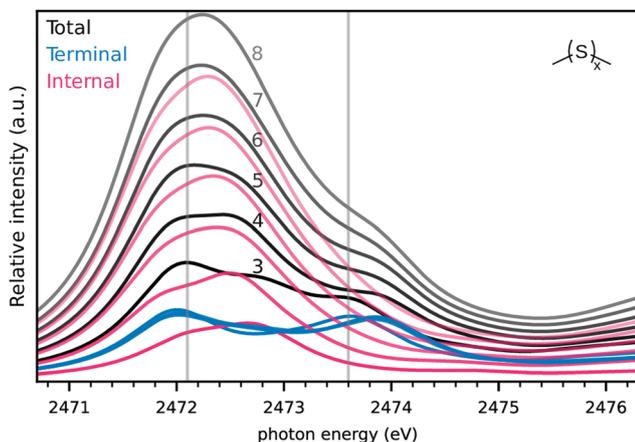
Fig. 5 NEXAFS spectra of di-methyl  $S_x$ -strands ( $DMS_x$ ) with  $x = 3$  to 8. The black lines are the total spectra of all S atoms, contributions from internal S atoms shown in magenta, and from terminal S atoms in blue.
