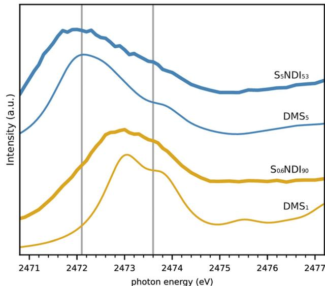
Fig. 6 *In situ* S-NEXAFS on cathodes with NDI crosslinker are shown in thick lines.  $S_{0.6}NDI_{90}$  and  $S_5NDI_{53}$  are two cathodes of varying S-content, with the subscript to S indicating the nominal average S-rank, and the subscript to NDI indicating its weight per cent. Thin lines: simulated spectra of dimethyl sulfide ( $DMS_1$ ) and dimethyl pentasulfide ( $DMS_5$ ).
