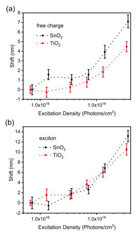
Fig. 6 Edge shifts of the FAPbBr<sub>3</sub>/ETL films at various excitation densities and the reference sample was measured under the lowest excitation density: (a) Left edge and (b) right edge.
