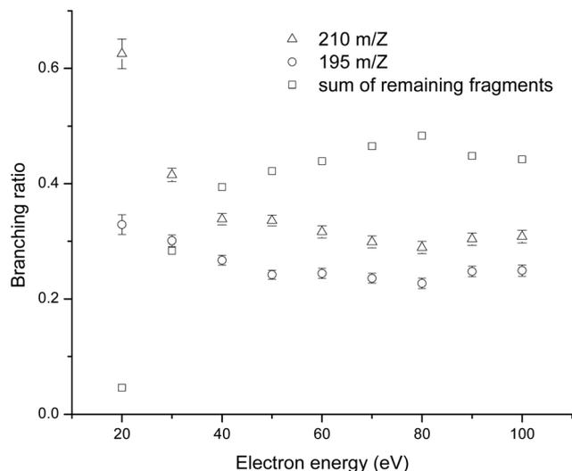
Fig. 3 Electron energy dependency of the branching ratios for  $m/z$  210, parent cation (triangles),  $m/z$  195, demethylated parent cation (circles), and the sum of all remaining fragments (squares), from 20 to 100 eV, in 10 eV steps.
