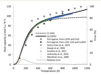
Fig. 2 Heat capacity of LiCoO<sub>2</sub> and comparison with experimental measurements. $^{10-14}$  A fit of experimental data was used to calculate the relative error of the calculated  $C_p$ . Two Neumann-Kopp approximations were derived: from  $\text{Li}_2\text{O}_2$  + CoO and from  $\text{Li}_2\text{O}$  + CoO + Co<sub>3</sub>O<sub>4</sub>. 96
