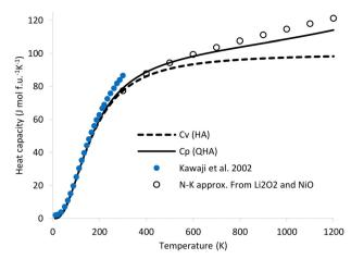
Fig. 3 Heat capacity of LiNiO<sub>2</sub> and comparison with experimental data<sup>18</sup> and with a Neumann–Kopp approximation from oxides  $\mathrm{Li_2O_2}$  and  $\mathrm{NiO.}^{96}$
