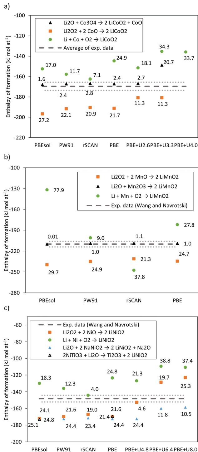
**Fig. 1** Formation energy of (a) LiCoO<sub>2</sub> (b) o-LiMnO<sub>2</sub> and (c) LiNiO<sub>2</sub> according to the DFT-computed reaction and the x-c functional. The dashed line is the experimental value. The numbered label on each point is the absolute value of the energy difference between the result and the experimental value.<sup>10,15–17,33</sup> The dotted lines represent the precision threshold level of  $\pm 4$  kJ mol<sup>-1</sup> for CALPHAD applications.
