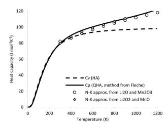
Fig. 4 Heat capacity of o-LiMnO2 in P2/c symmetry calculated with a QHA from Fleche<sup>47</sup> and comparison with a two Neumann-Kopp approximation: from  $Li_2O + Mn_2O_3$  and from  $Li_2O_2 + MnO.$ <sup>57,96,99</sup>
