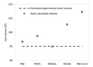
Fig. 5 Calculated cell volume of LiCoO<sub>2</sub> for different x-c and comparison with an estimated experimental static volume derived from ref. 50.
