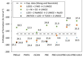
Fig. 1 Formation energy of (a) LiCoO $_2$  (b) o-LiMnO $_2$  and (c) LiNiO $_2$  according to the DFT-computed reaction and the x-c functional. The dashed line is the experimental value. The numbered label on each point is the absolute value of the energy difference between the result and the experimental value.  $^{10.15-17.33}$  The dotted lines represent the precision threshold level of  $\pm$  4 kJ mol at  $^{-1}$  for CALPHAD applications.
