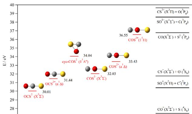
Fig. 3 [O,C,S] sum formula doubly charged minimal structures as computed at the RCCSD(T)/aug-cc-pV(Q+d)Z level of theory. We locate the [CO + S]<sup>2+</sup>, [SO + C]<sup>2+</sup> and [CS + O]<sup>2+</sup> channels, where the fragments are in their ground states. These energies are given with respect to the neutral OCS (X<sup>1</sup>Σ<sup>+</sup>) ground state. The ZPE correction is also included. See Tables S1–S3 (ESI†) for more details.
