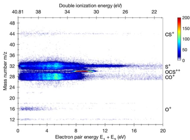
Fig. 1 Electron–electron–ion coincidence map for OCS obtained at a photon energy of  $h\nu = 40.81$  eV in the form of mass number against summed electron pair energy on the bottom axis and double ionization energy on the top axis.
