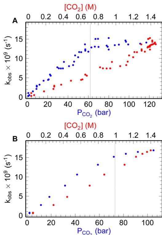
Fig. 2 The  $e_{\text{hyd}}^-$  decay rate (blue dots) at different pressures and concentrations of  $\text{CO}_2$  (red dots): A – for 25 °C; B – for 35 °C.
