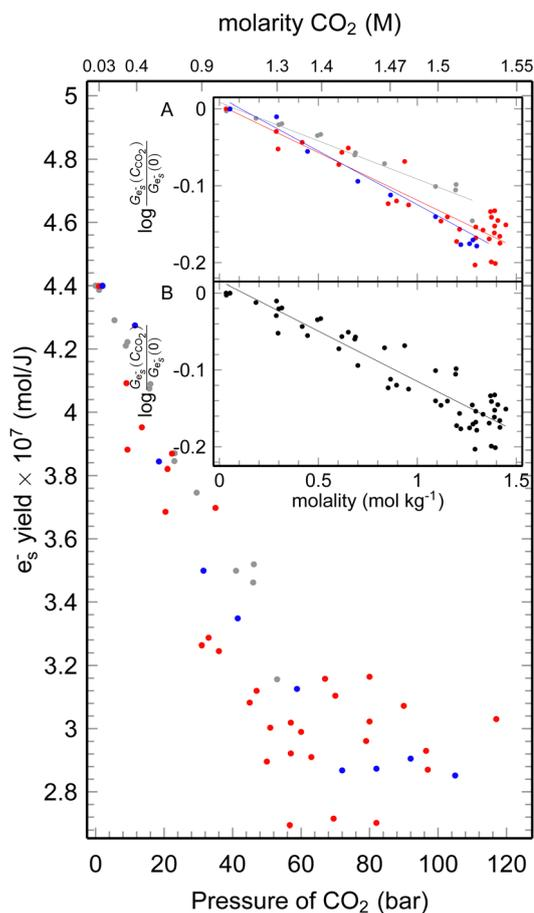
Fig. 3 The yield of  $e_{\text{hyd}}^-$  at 10 ps after the 7 ps electron pulse at different  $\text{CO}_2$  pressures, the gray dots data up to 51 bars;<sup>4</sup> red dots – data at 25 °C, blue dots – data at 35 °C. Inset: Plot of the  $e_{\text{hyd}}^-$  yield fraction remaining vs. the concentration of the  $\text{CO}_2$  A – 25 °C, B – 35 °C.
