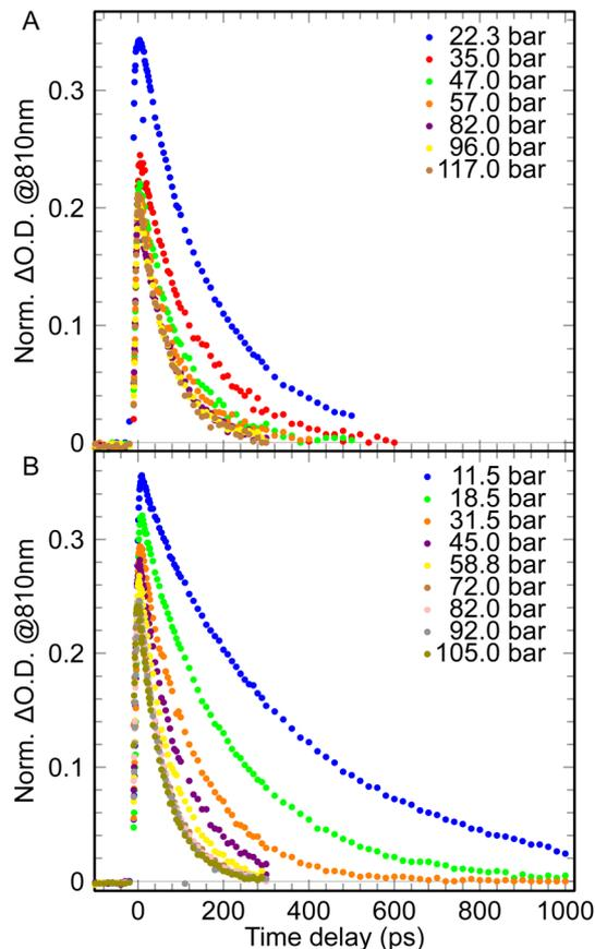
Fig. 1 The pulse radiolysis data of a water-CO<sub>2</sub> system at different pressures for nanosecond timescale: A – for 25 °C; B – for 35 °C.
