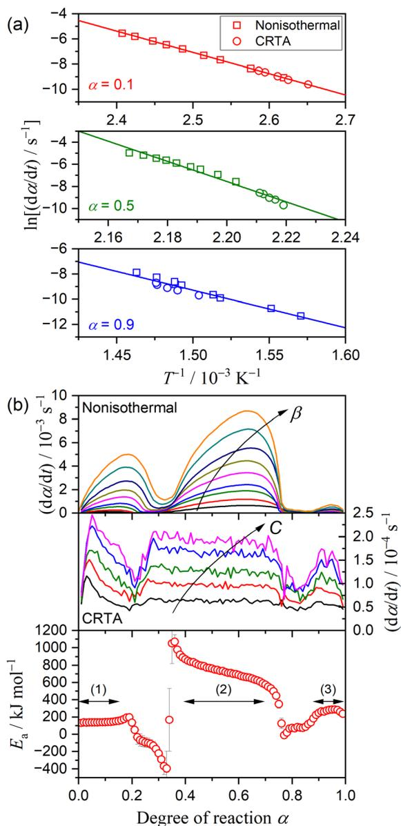
Fig. 4 Results of isoconversional kinetic analysis for the overall thermal dehydration of DCPD (63–75  $\mu m$ ) in a stream of dry  $N_2$ : (a) Friedman plot at different  $\alpha$  values, and (b) changes in  $(d\alpha/dt)$  as the reaction advances under linear nonisothermal and CRTA conditions, and  $E_a$  values at different  $\alpha$ .
