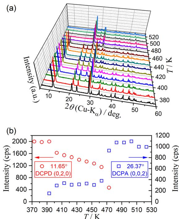
Fig. 11 Change in the XRD pattern of DCPD (63–75  $\mu\text{m}$ ) during the stepwise isothermal heating in a stream of dry  $\text{N}_2$ : (a) XRD patterns at different temperatures, and (b) variation in the intensity of selected diffraction peaks of DCPD at (0, 2, 0) and DCPA at (0, 0, 2).
