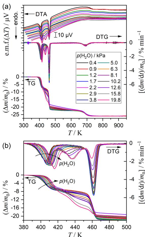
**Fig. 7** (a) TG–DTG–DTA curves for the thermal dehydration of DCPD (63–75  $\mu\text{m}$ ;  $m_0 = 5.00 \pm 0.03$  mg) at a  $\beta$  of  $5 \text{ K min}^{-1}$  and (b) a view focused on the thermal dehydration of DCPD to form DCPA.
