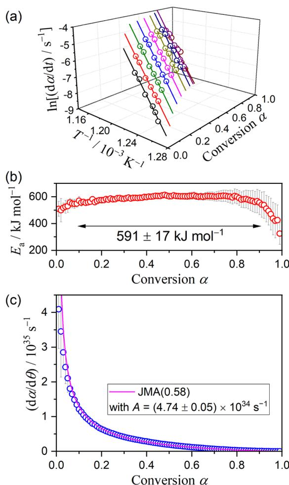
Fig. 16 Results of the formal kinetic analysis for the crystal growth of  $\gamma$ -CPP: (a) Friedman plot at various  $\alpha$ , (b)  $E_a$  values at different  $\alpha$ , and (c) experimental master plot and fit curve using JMA(0.58).
