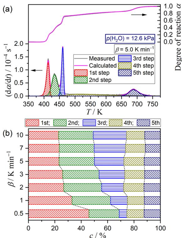
Fig. 9 Results of KDA for the multistep thermal dehydration of DCPD (63–75  $\mu\text{m}$ ) in a stream of  $\text{N}_2$ – $\text{H}_2\text{O}$  mixed gas with  $p(\text{H}_2\text{O}) = 12.6$  kPa: (a) typical fitting results for the overall reaction under linear nonisothermal conditions at a  $\beta$  of  $5 \text{ K min}^{-1}$  and (b) contributions of individual steps at various  $\beta$  values.
