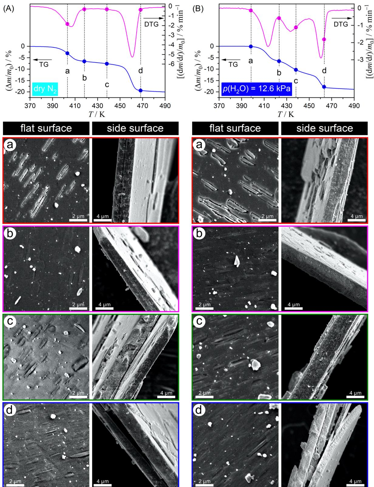
Fig. 12 Changes in the surface morphology of sample particles during the thermal dehydration of DCPD (63–75 μm) to form DCPA in a stream of dry N<sub>2</sub> (A) and N<sub>2</sub>-H<sub>2</sub>O mixed gas with  $p(\text{H}_2\text{O}) = 12.6$  kPa (B): (A)-a: 403 K; (A)-b: 418 K; (A)-c: 438 K; (A)-d: 468 K; (B)-a: 398 K; (B)-b: 423 K; (B)-c: 438 K; (B)-d: 463 K.
