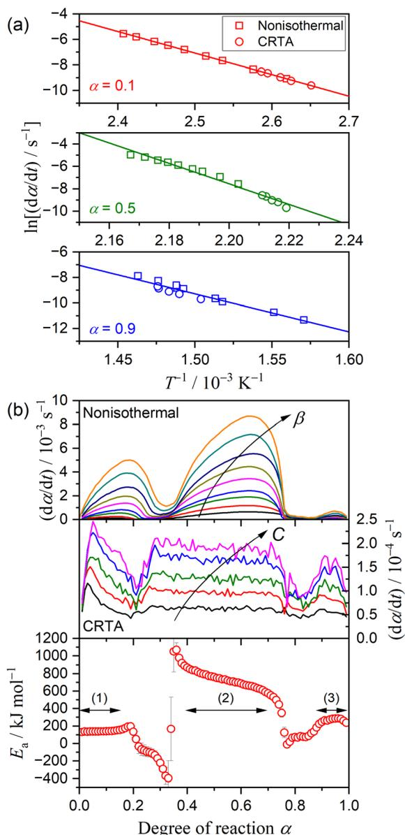
Fig. 4 Results of isoconversional kinetic analysis for the overall thermal dehydration of DCPD (63–75  $\mu\text{m}$ ) in a stream of dry  $\text{N}_2$ : (a) Friedman plot at different  $\alpha$  values, and (b) changes in  $(d\alpha/dt)$  as the reaction advances under linear nonisothermal and CRTA conditions, and  $E_a$  values at different  $\alpha$ .
