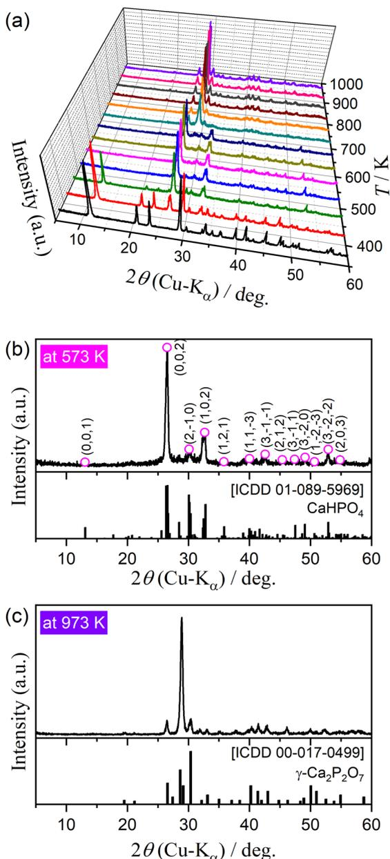
Fig. 2 Change in the XRD pattern of DCPD sample (63–75  $\mu\text{m}$ ) during stepwise isothermal heating in a stream of dry  $\text{N}_2$ : (a) XRD patterns at different temperatures, (b) XRD pattern at 573 K, and (c) XRD pattern at 973 K.
