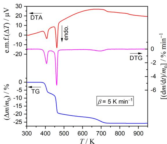
Fig. 1 TG-DTG-DTA curves recorded during the heating of DCPD sample (63–75 μm;  $m_0 = 4.99$  mg) from 300 K to 973 K at a  $\beta$  of 5 K min<sup>-1</sup> in a stream of dry N<sub>2</sub> ( $q_v = 300$  cm<sup>3</sup> min<sup>-1</sup>).
