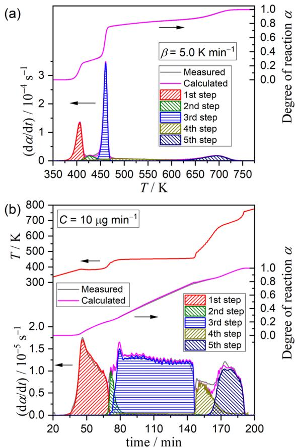
Fig. 5 Typical fitting results of KDA for the partially overlapping five-step mass loss process of the thermal dehydration of DCPD (63–75  $\mu\text{m}$ ) in a stream of dry  $\text{N}_2$  under different heating program modes: (a) linear nonisothermal at  $\beta = 5 \text{ K min}^{-1}$  and (b) CRTA at  $C = 10 \mu\text{g min}^{-1}$ .
