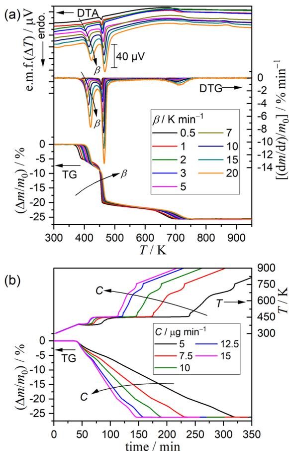
Fig. 3 TG-DTG-DTA or TG-temperature profile curves recorded during heating of DCPD sample (63–75  $\mu\text{m}$ ) in a stream of dry  $\text{N}_2$  with different temperature program modes: (a) linear nonisothermal mode at different  $\beta$  values ( $m_0 = 5.00 \pm 0.03$  mg) and (b) CRTA mode at different  $C$  values ( $m_0 = 5.00 \pm 0.04$  mg).
