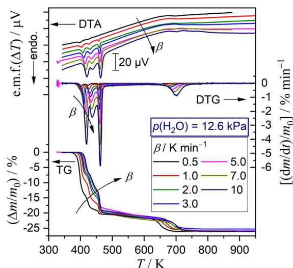
**Fig. 8** TG–DTG–DTA curves for the thermal dehydration of DCPD (63–75  $\mu\text{m}$ ;  $m_0 = 5.03 \pm 0.07$  mg) at different  $\beta$  values in a stream of  $\text{N}_2$ – $\text{H}_2\text{O}$  mixed gas ( $q_v = 200 \text{ cm}^3 \text{ min}^{-1}$ ) with  $p(\text{H}_2\text{O}) = 12.6$  kPa.
