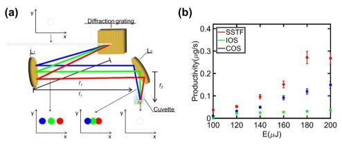
Fig. 6 (a) Experimental setup of the fs SSTF-PLAL system based on the spatial separation of the spectral components of an fs pulse that is only recombined at the focal spot, returning to the initial fs pulse duration. (b) NP productivity as a function of the pulse energy for the fs SSTF-PLAL, standard fs PLAL (COS), and analogous system to fs SSTF-PLAL without spatial separation of the spectral components (IOS). Reproduced from ref. 99 with permission from Chinese Laser Press, copyright 2019.
