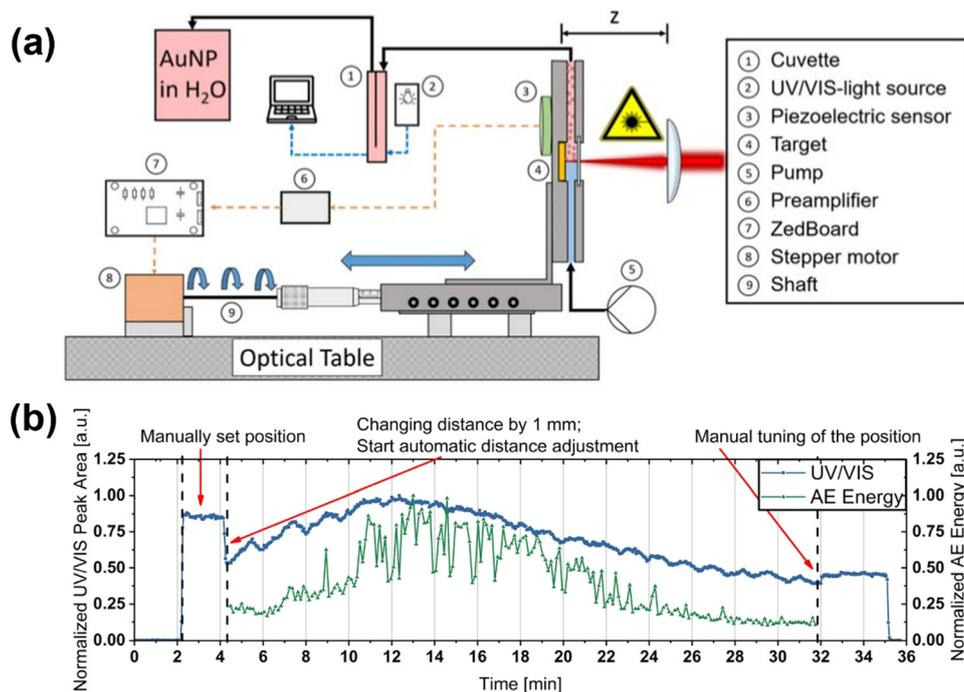
Fig. 16 Real-time monitoring and automatic control of the working distance in the PLAL system, where (a) shows the experimental set-up and (b) shows the comparison between the acoustic emission (AE) signal and UV-Vis spectra over time. Adapted from ref. 167 with permission from Elsevier, copyright 2019.
