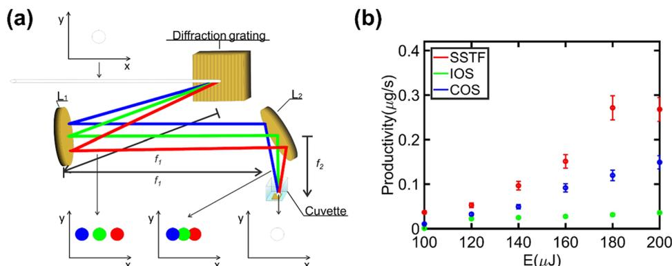
Fig. 6 (a) Experimental setup of the fs SSTF-PLAL system based on the spatial separation of the spectral components of an fs pulse that is only recombined at the focal spot, returning to the initial fs pulse duration. (b) NP productivity as a function of the pulse energy for the fs SSTF-PLAL, standard fs PLAL (COS), and analogous system to fs SSTF-PLAL without spatial separation of the spectral components (IOS). Reproduced from ref. 99 with permission from Chinese Laser Press, copyright 2019.
