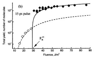
Fig. 3 Simulation of laser ablation of organic solids at different fluences using two different pulse widths. Hollow data points represent the ablation regime below the ablation threshold and the filled data points denote the ablation at or above the ablation threshold. The graphs show that the ablation using a shorter pulse width resulted in a lower ablation threshold fluence. Reproduced from ref. 106 with the permission from AIP Publishing, copyright 2000
