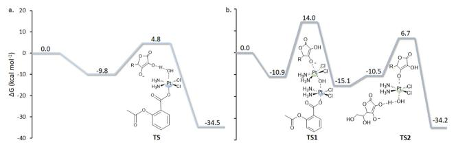
Fig. 3 Reduction mechanism following mechanism (b), the shift of a hydride ( $H^-$ ) unit from the OH group of the ascorbate to the hydroxido ligand (panel a), and the  $Pt^{II}$ -catalyzed mechanism (d) (panel b).
