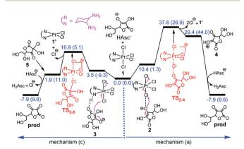
Fig. 1 Free energy profiles describing the reduction of the tetraplatin complex by AscH- via inner sphere mechanisms (a) and (c) in water. In parentheses, electronic energies are provided. Adapted from ref. 41 with permission. Copyright 2017 by The Royal Society of Chemistry
