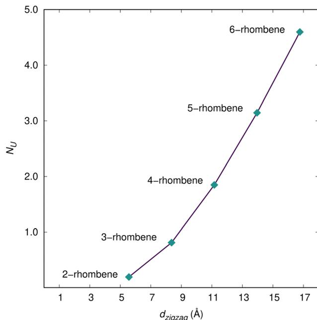
Fig. 2 Evolution of the  $N_U$  values of  $n$ -rhombenes, as calculated by the FT-TPSS/def2-TZVP method, as a function of the zigzag length (in Å) measured as the sum of the  $(2n)$  CC bond lengths along one of the four (symmetrical) edges of the systems.
